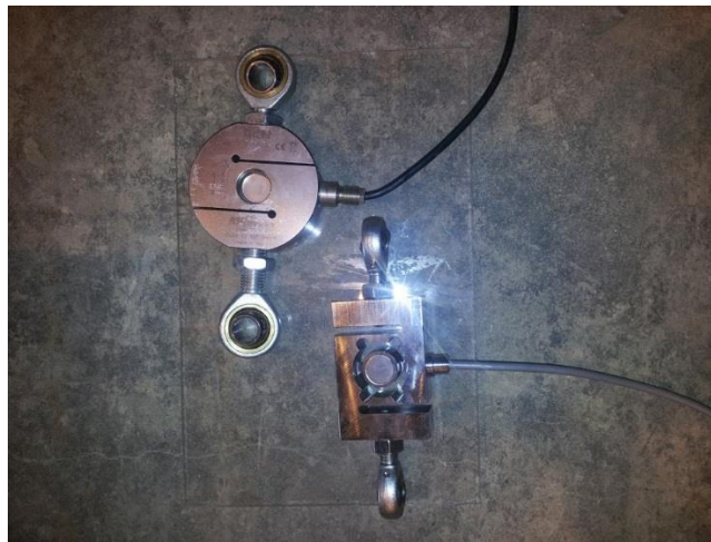
Figure 32: 2000 kg (upper left) and 200 kg (lower right) load cells/tension meters
