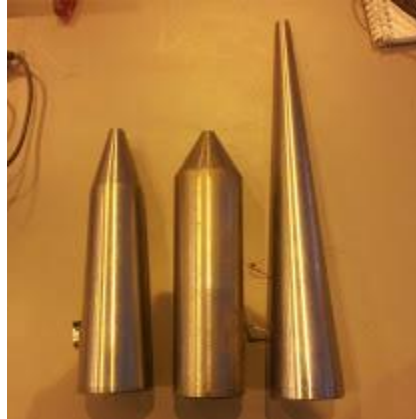
Figure 33: BHAs milled in the workshop. From left to right: BHA 3, BHA 1, and BHA 2
