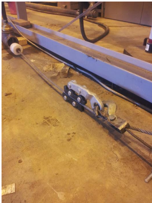
Figure 30: Jack and tighten clamp attached to drillstring to free stuck BHA
