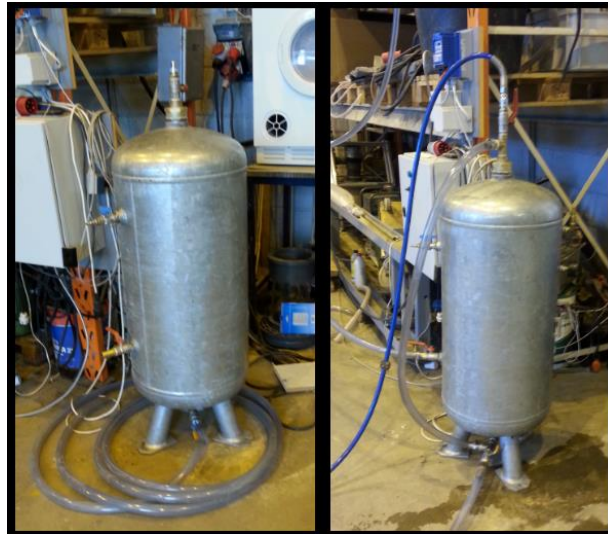
Figure 5.10 Pressure tank used to displace mud. To the right a tube has been installed to see the fluid level inside the tank. To the right we also see a blue hose filling the tank up with air used to increase pressure in the tank.
