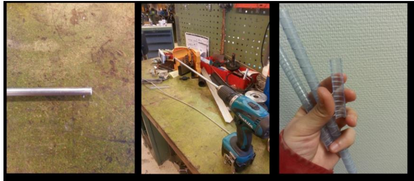
Figure 5.7 A nail attached to a pole was run through the pipes and created desired internal roughness
