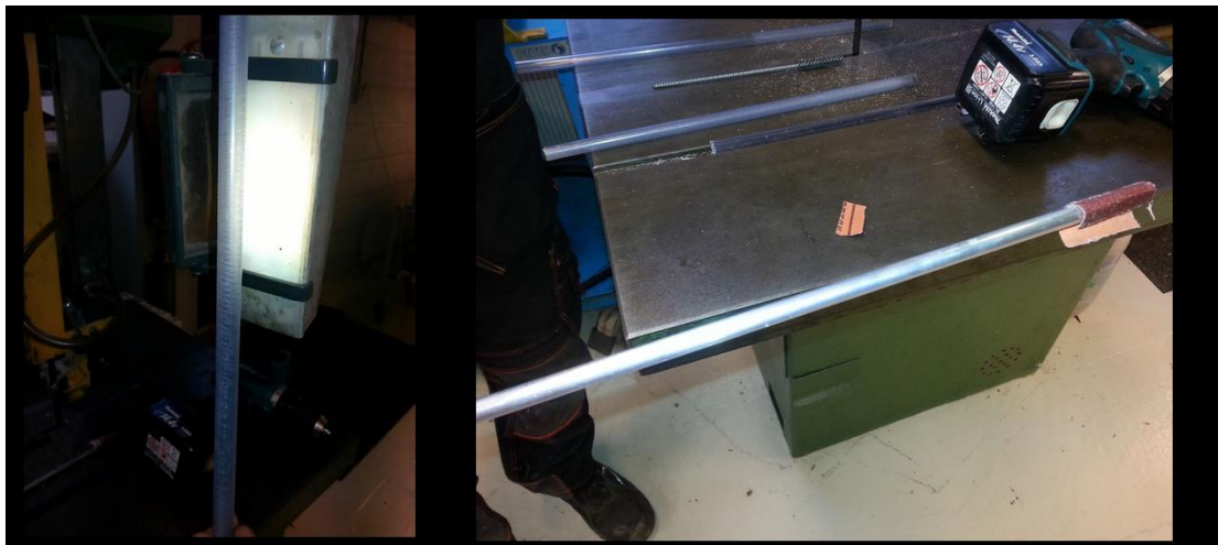
Figure 5.4 Trying to create internal roughness with sandpaper. This did not create enough internal roughness in the pipes.
