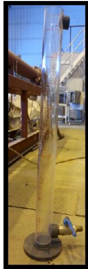
5.11: A Measurement Cylinder was used to measure how much oil and displacement fluid was displaced after each test.
