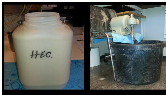
5.14: HEC is a viscous fluid. Mixed with water, it will give us the needed viscosity and density to analyze effects of viscosity and density of the displacing fluid has on displacement.
