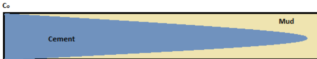
Figure 4.2: Velocity Profile of the Cement after x seconds. There is still no slip of cement at the walls.
