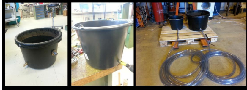
Figure 5.9 Two tanks intended for containing the oil and displacement fluid were drilled and we attached tubes to them. Pressure from the tanks was going to be provided through a height difference created when the tanks were lifted up. This was not safe, so the tank containing displacement fluid was switched to a pressure tank. The tank containing oil was placed in fixed place at 3 meters above the pipe.
