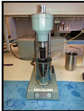
Figure 5.15: Viscosity meter used to take correct measurements of the viscosity in the viscous fluids used to displace oil.
