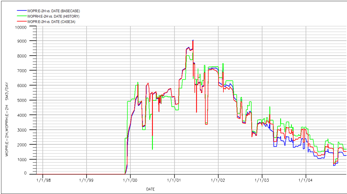
Figure 5.2.3.20 Well E-2H OPR Green=History Data, Blue=Basecase Model Data, Red= History Matched data
