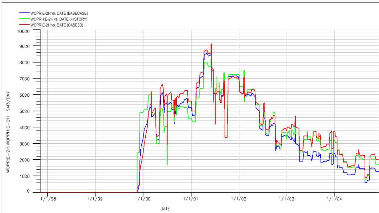
Figure 5.2.3.29 E-2H Oil production rate, Green=History Data, Blue=Basecase Model Data, Red= History Matched data
