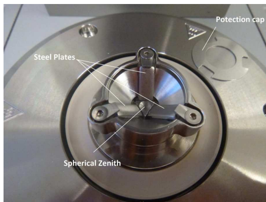
Figure 3.3: Three steel plates in the friction apparatus of the MCR.
