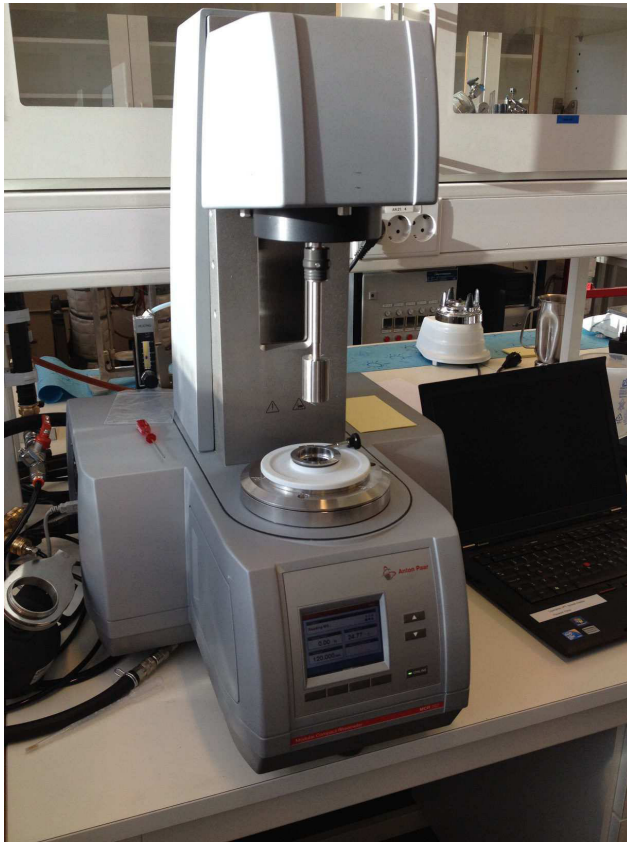
Figure 3.5: Modular Compact Rheometer (MCR) with mounted viscometer measurement equipment. The viscometer is visible as the bob and cup part of the MCR apparatus.
