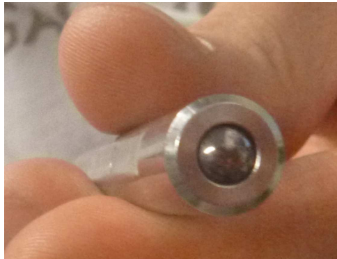
Figure 4.4: Illustration of the pin with a ball mounted to the bottom
