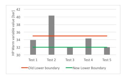
Figure 6.13: HP Warm value after reducing lower boundary Turbo-expander process
