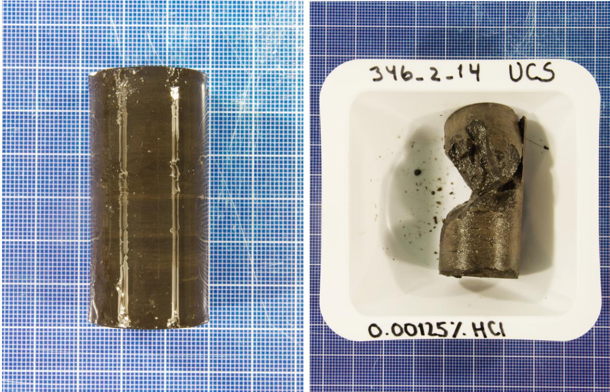
Figure III- 6: Core sample 346_2_14 before and after failure.
