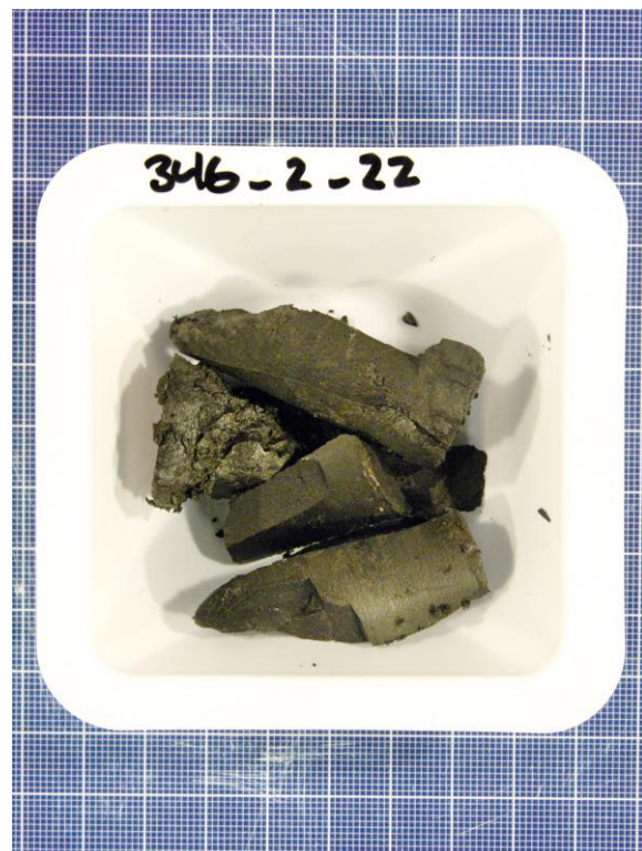
Figure XI- 6: Core sample 346_2_22 after creep test.
