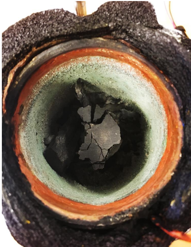
Figure XII- 4: Dried out core sample inside container due to leakage/evaporation of fluid.
