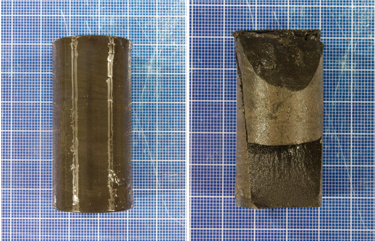
Figure III- 8: Core sample 346_2_16 before and after failure.
