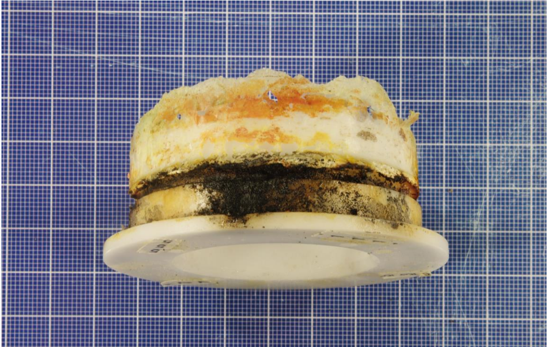
Figure XII- 3: Melted plastic parts from the experimental setup.
