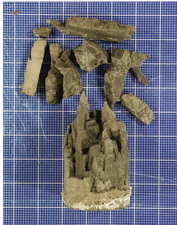
Figure XI- 4: Core sample 346_2_20 after creep test.
