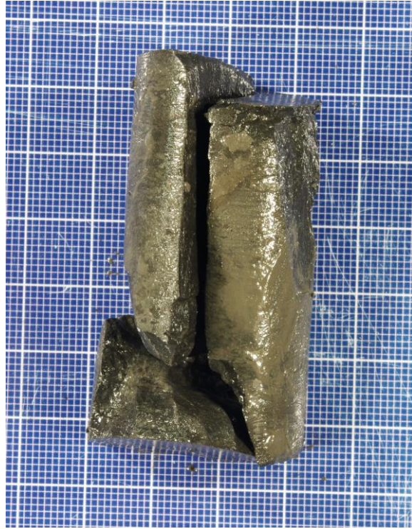
Figure XI- 3: Core sample 346_2_19 after creep test.
