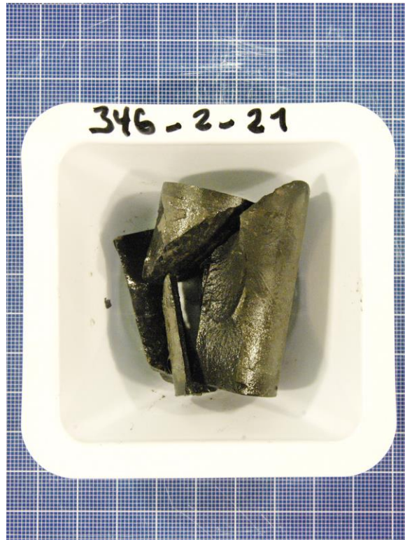
Figure XI- 5: Core sample 346_2_21 after creep test.
