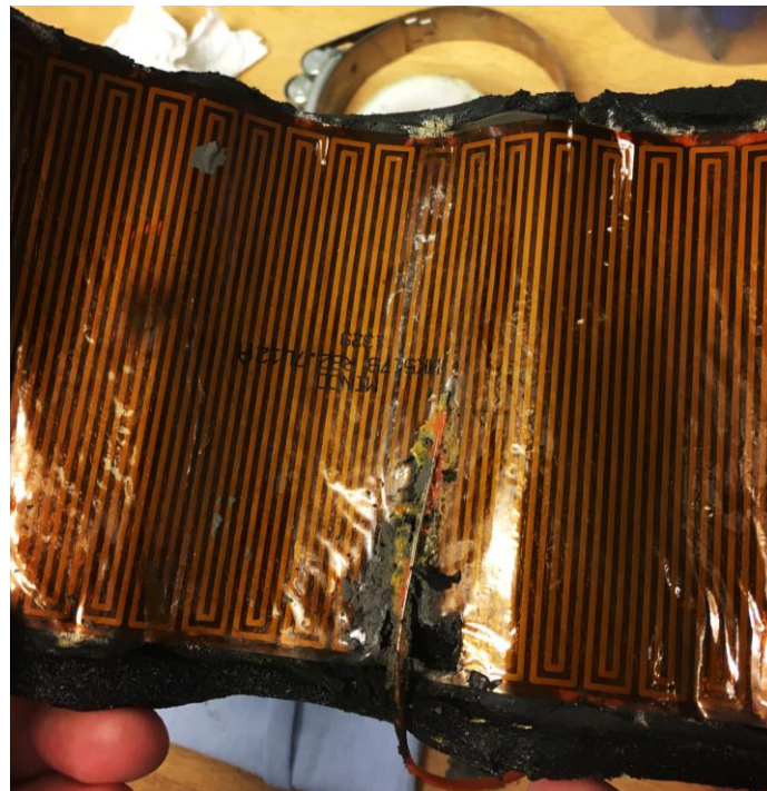
Figure XII- 1: A damaged heating element.
