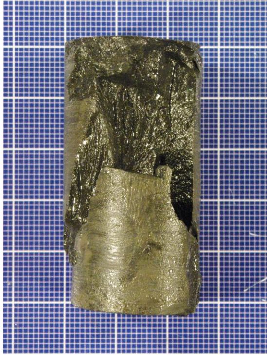
Figure XI- 7: Core sample 346_2_23 after creep test.
