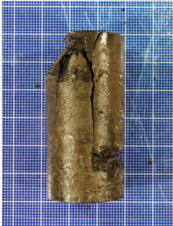
Figure XI- 1: Core sample 346_2_15 after creep test.
