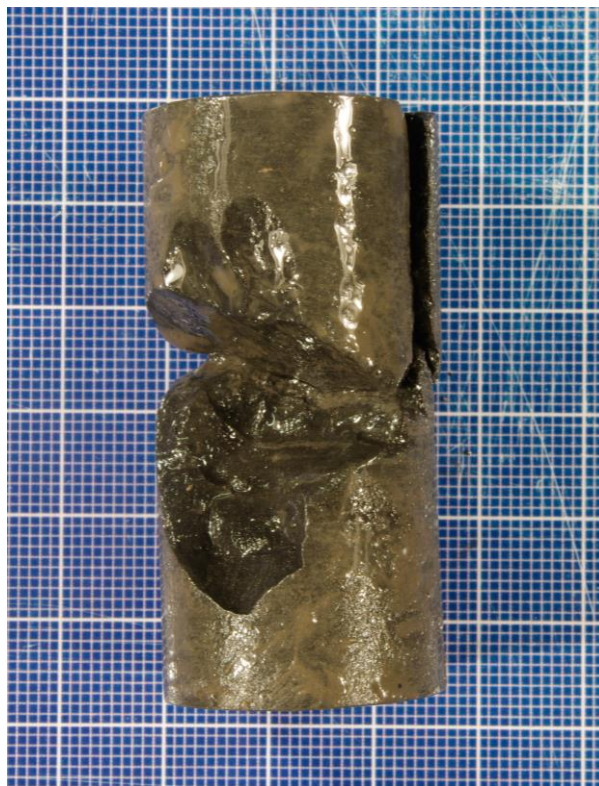
Figure XI- 2: Core sample 346_2_18 after creep test.
