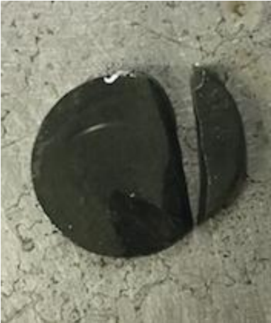
Figure G- 2 Disintegrated shale sample caused by the exposure to hydrochloric acid
