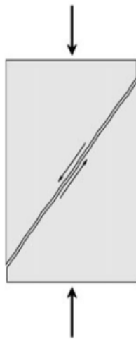
Figure 3- 2 Shear failure (Fjær et al., 2008)
