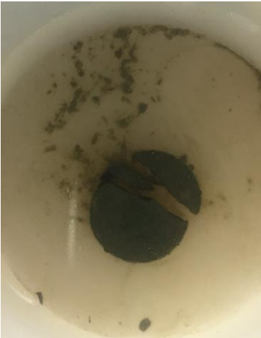
Figure G- 3 Disintegrated shale sample caused by the exposure to brine. The surface of the sample is crumbled.
