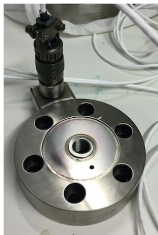
Figure 4- 12 Load cell recording the total axial force applied to the load frame
