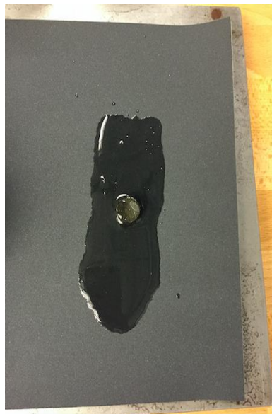
Figure 4- 6 Grinding process during sample preparation
