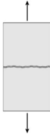
Figure 3-1 Tensile failure (Fjær et al., 2008)
