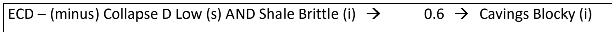
Figure 4-3: An AND relationship. Shale Brittle (i) is required on the left side for ECD - Collapse D Low (s) to relate to Cavings Blocky (i). The relation-strength is 0.6.
