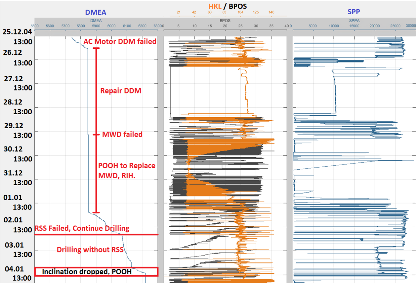
Figure 7-15: One-week summary of RTDD prior to failure. Explanation of important events were added in red. The point of failure occurred at 13:00. (Raknes, 2014), free after (Operator, RTDD, 2005)
