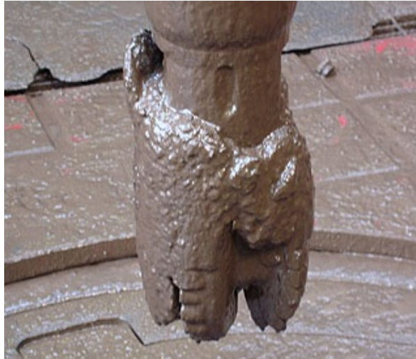
Figure 3: Accumulated materials within the cutting structure of the bit (Drillingformulas 2014).
