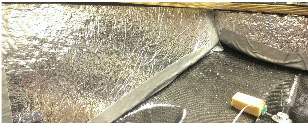
Figure 3.3: The inside of the hull with noise reduction mat.
