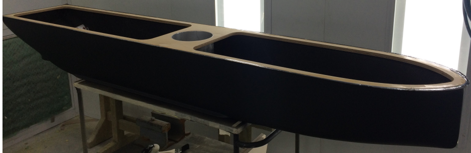
(a) After epoxy curing process.
