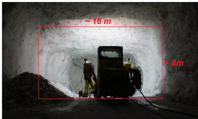
Figure 5.3: Approximate dimensions of drifts in the mine
