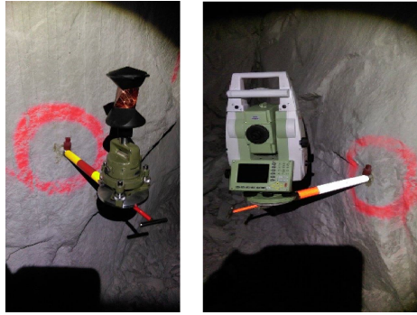
Figure 5.5: The equipment used during the measurement on the known points
