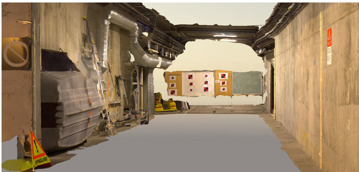
Figure 4.11: 3D mesh model produced from photos captured with Sony provided by Context Capture
