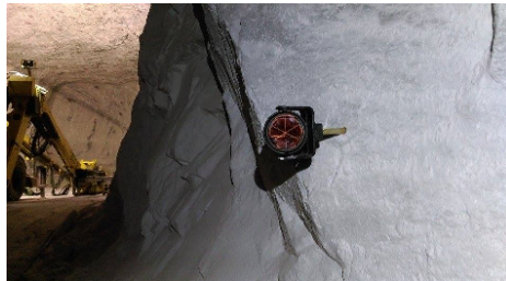
Figure 5.6: The fix point with the prism mounted on the bolt
