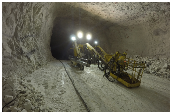
Figure 5.9: The mobile drilling rig with LED lamps
