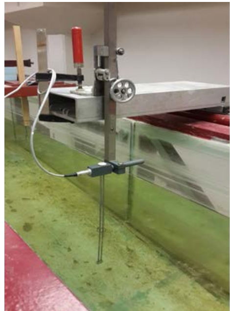
(b) Wave gauge used in the experiment
