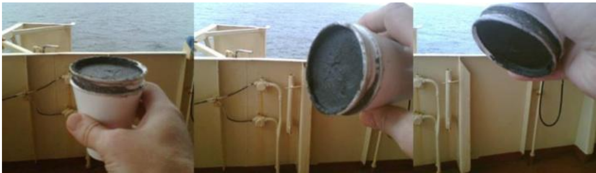
Figure 3.2: Sandaband (Sandaband Well plugging, 2012)
