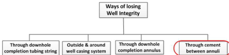
Figure 2.4: Ways of losing well integrity. Red ring shows the focus of this thesis
