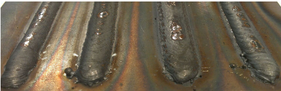
(b) Feed speed 6.0 m/min. Amplitude: 2 - 4 - 5 - 4 [mm]. Weave pattern: TW - TW - TW - SW
