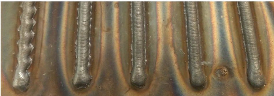
(b) Triangle weave, amplitude = 2mm. From left to right: 0.5 - 1.0 - 1.5 - 2.0 - 2.5 [Hz]
