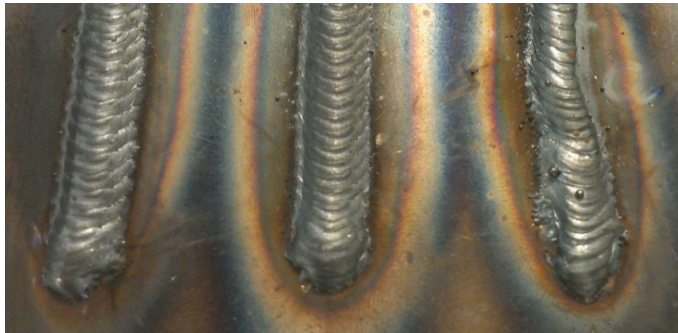
(a) Triangle weave, amplitude = 4mm. From left to right: 1.25 - 1.5 - 1.75 [Hz]
