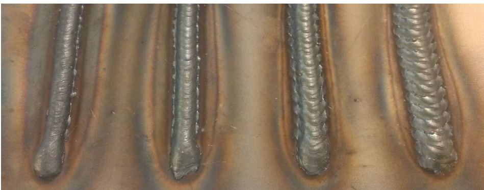
Figure 5.5: Preliminary plate tests: Various amplitude at 1 Hz triangle weave. From left to right: 1.0 - 2.0 - 3.0 - 4.0 [mm]
