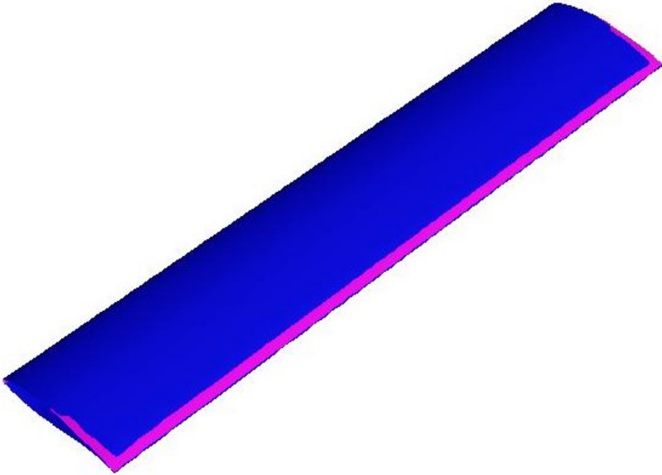
Figure 5.5: x-wall shear stress over the top of the airfoil for double domain dimensions. Separation marked in pink
