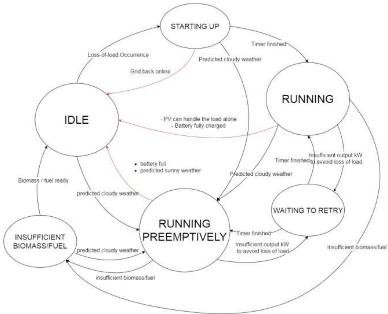
Figure 2:26 Biomass System State-Machine Transition Diagram
