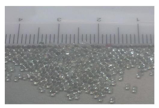
Figure 25. Non-spherical particle used during experimental investigation (d=3.387mm)
