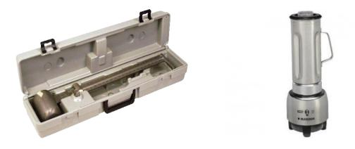
Figure 9. a) Mud balance (left)(Anony. 2013) and b) Waring laboratory blender(right)(Anon 2013).
