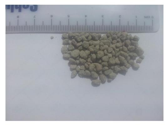
Figure 27. Non-spherical particle used during experimental investigation (d=3.387mm)
