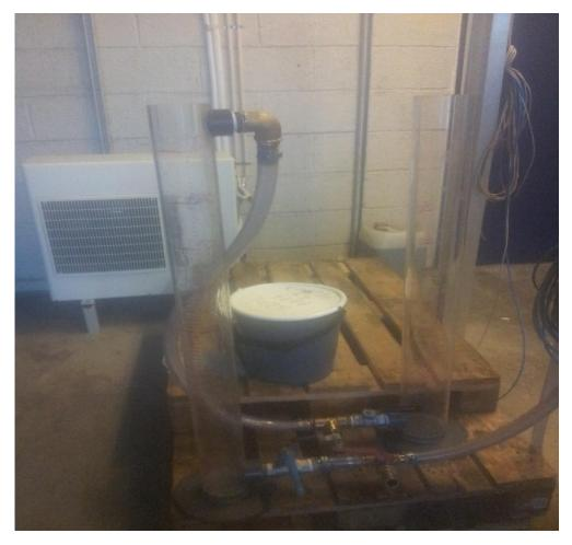
Figure 24. Experimental device used for investigation of particle slip velocity under steady state laminar flow
