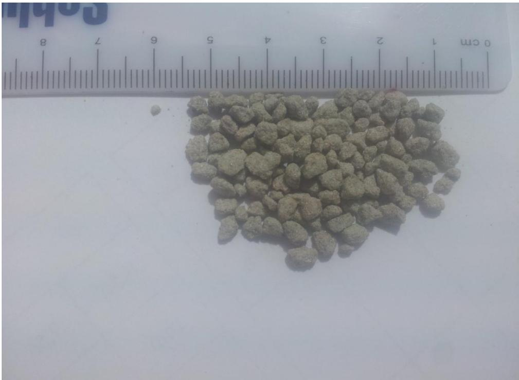
*Figure 27. Non-spherical particle used during experimental investigation ( $d=3.387\text{mm}$ )*
