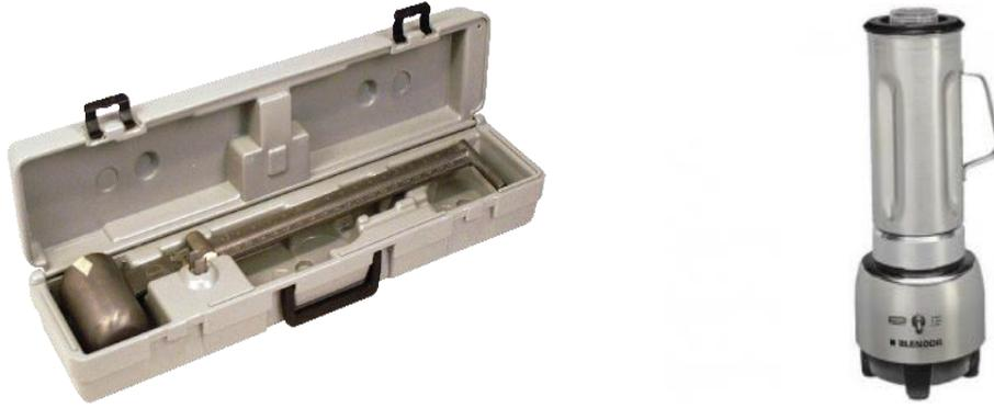
*Figure 9. a) Mud balance (left)(Anony. 2013) and b) Waring laboratory blender(right)(Anon 2013).*
