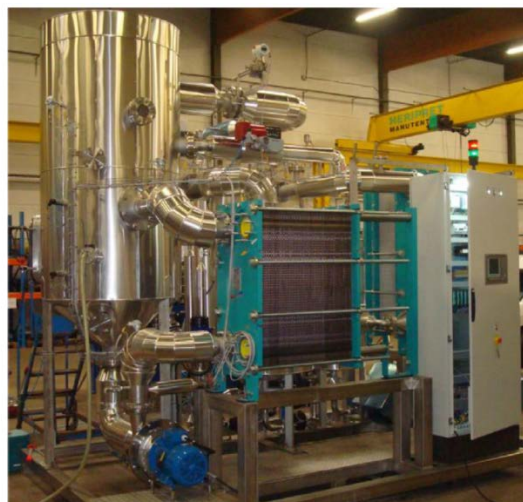
Figure 3.1 Prototype heat pump with water as refrigerant (Chamoun et al., 2014).
