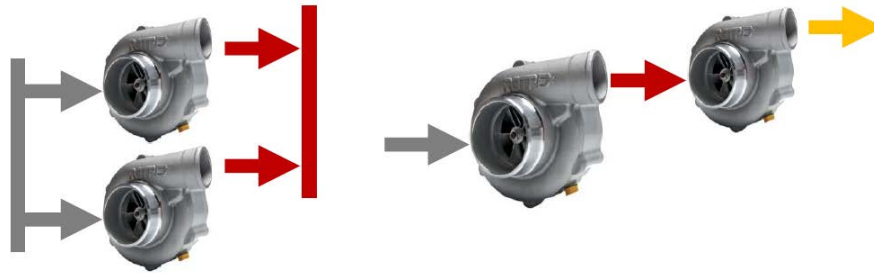
Figure 3.2 Compressor set up in parallel combined with serial coupling to achieve a higher temperature lift. (Madsboell et al., 2015)
