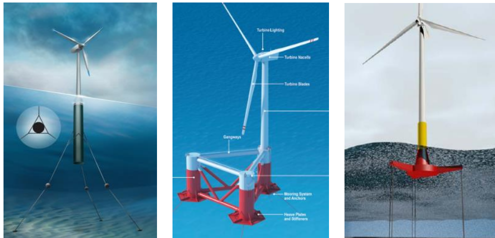
Figure 1-2: Floating wind turbine platforms (left to right: spar, semi-submersible, TLP)
