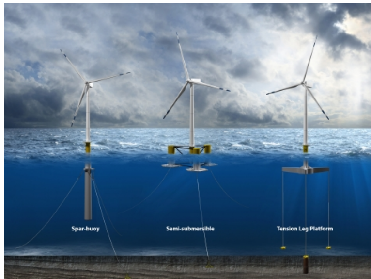
Figure 1.4: Concepts of floating wind turbine (left to right: Spar, Semi-submersible and TLP wind turbine concepts Matzat (2014) )
