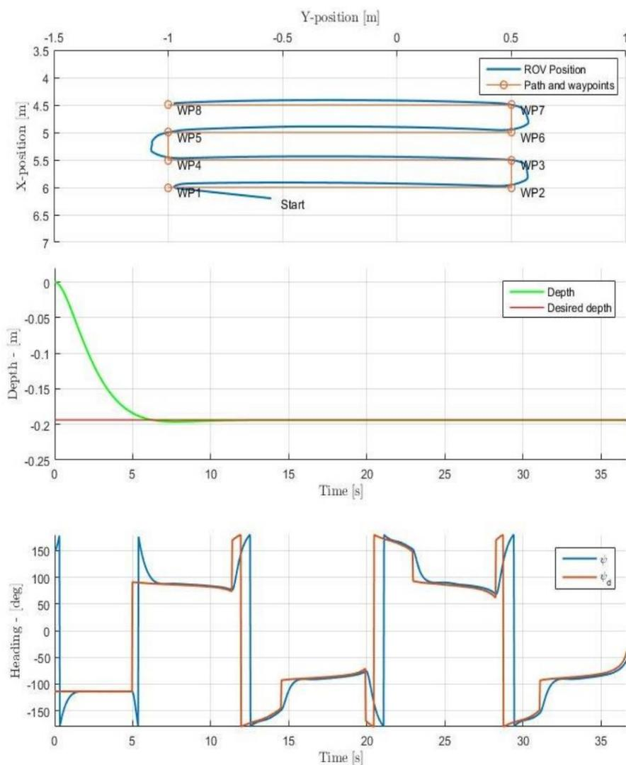
Simulation results verify that the mathematical model of the ROV is able to reach desired heading, depth and to follow the desired path with a very small error. When reaching the waypoint, the vessel will have a small velocity, resulting in an overshoot. Low-pass filters and saturating elements on the produced thruster forces are installed for more realistic and comparable results.
