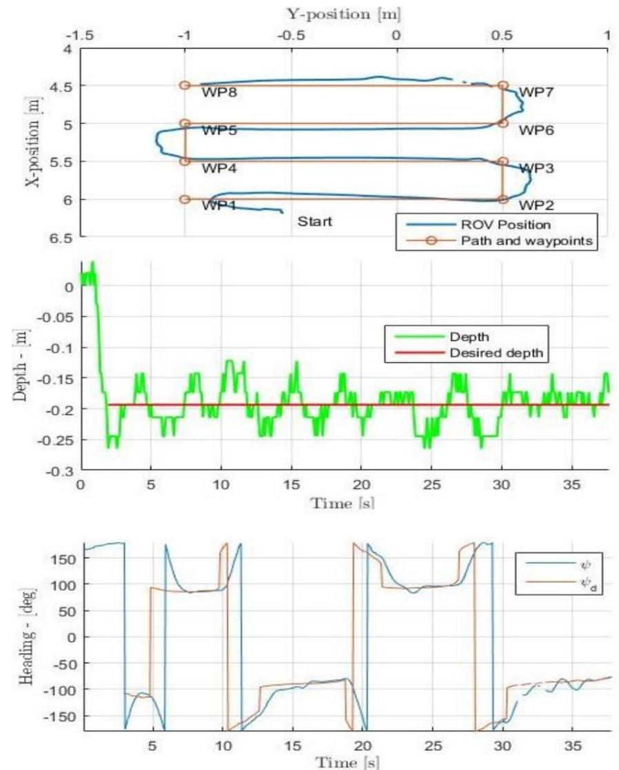
Results from experimental testing show that the ROV follows the path nicely. Position data are available throughout the entire run, except for a small time period after about 30 seconds, resulting in difficulties stabilizing the heading. Because no method for braking exists, the craft has a small velocity when reaching a waypoint, creating a small overshoot at the desired waypoints.
