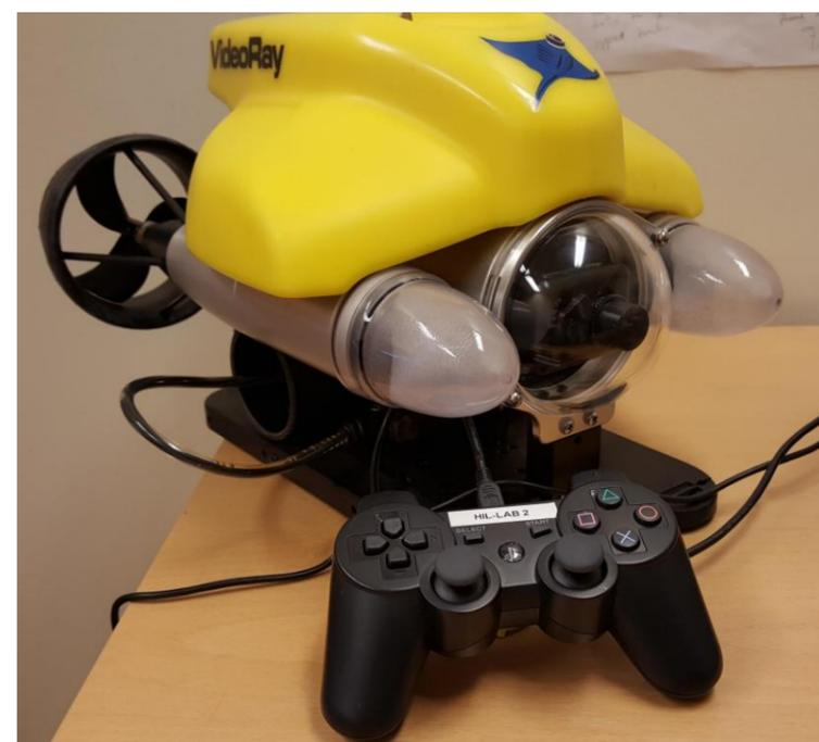
Communication with the ROV happens in C/C++ through an interface, called a mex-function, allows for code implementation, debugging and execution in Matlab directly. The ROV can be run on both Linux and Windows computers.
