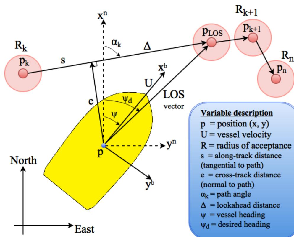
Taking a set of waypoints as input, the guidance system creates a path between each waypoint location. This path is followed by controlling adopting the LOS methodology and a technique for controlling thrust or velocity of the craft.
