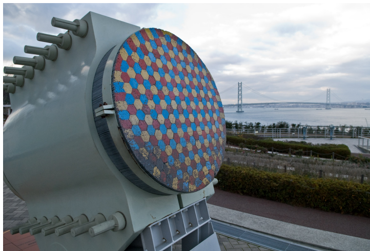
Figure 16: Example of cross section of a main cable used on suspension bridges
