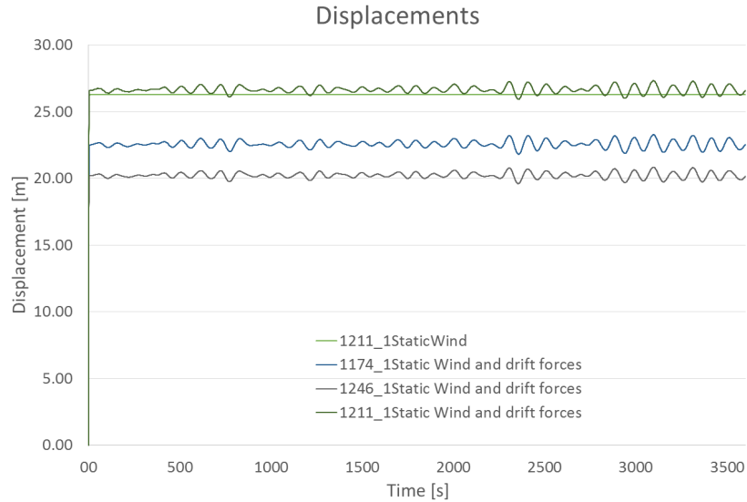
Figure 96: Response to mean wind and drift forces
