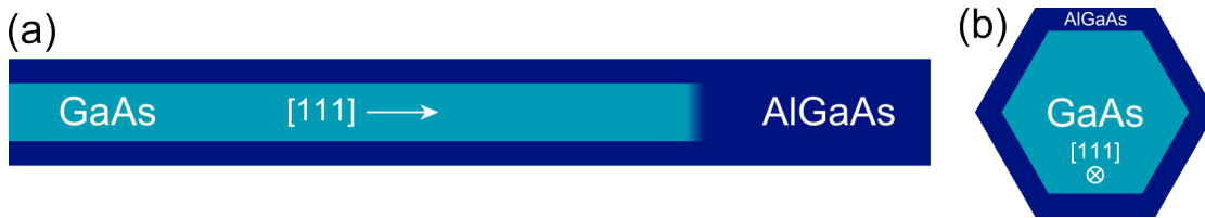
Figure 3.1: Schematic of a GaAs/AlGaAs core-shell nanowire.
