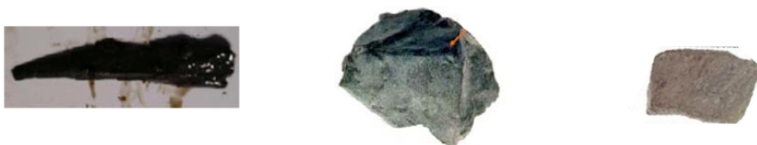
FIGURE 3.8: Different shape of the cuttings. To the left a splintery, the second is an angular and to the right is a blocky caving (Skalle 2011).
