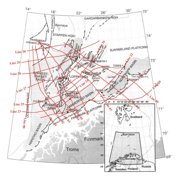
Figure 7: Map of seismic lines from MCG on top of structural elements in the southwestern Barents Sea. Modified from Gabrielsen and Kløvjan (1997) and MCG (2011).
