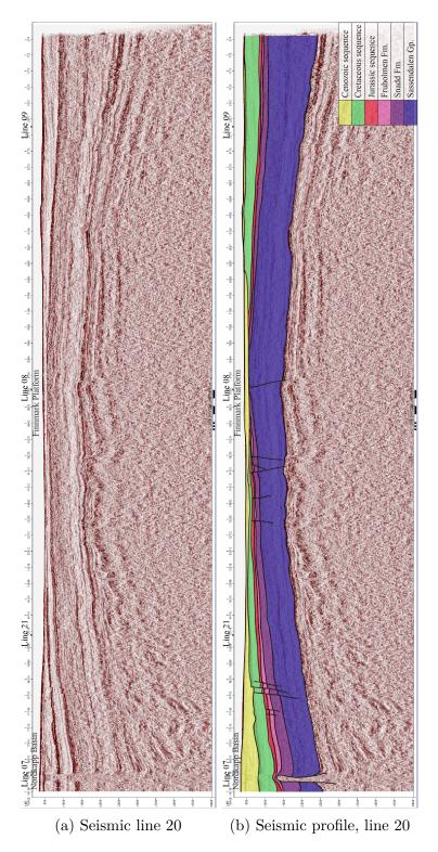
Figure 11: Seismic 2D line 20 and a profile showing the seismic interpretation. The location is shown in Figure 7.
