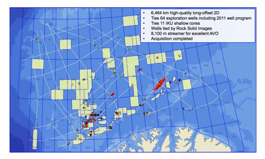
Figure 2: MCG's 2011 Barents Sea Supertie (MCG, 2011). The seismic 2D lines 00-09 are shot approximately SE-NW, and the lines 20-30 are shot approximately SW-NE.
