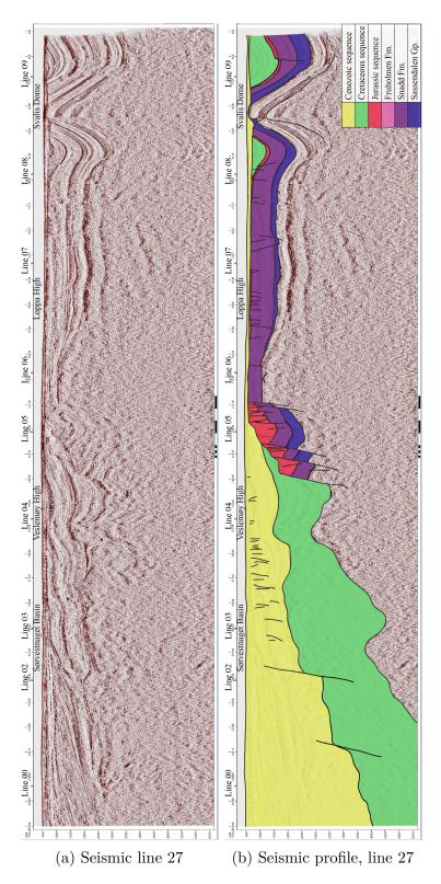
Figure 28: Seismic 2D line 27 and a profile showing the seismic interpretation. The location is shown in Figure 7. \$46\$
