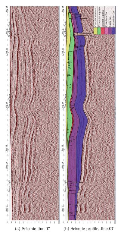
Figure 37: Seismic 2D line 07 and a profile showing the seismic interpretation. The location is shown in Figure 7.
