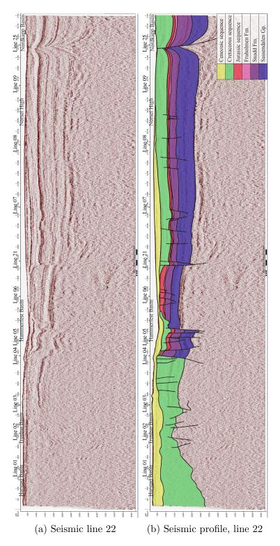
Figure 15: Seismic 2D line 22 and a profile showing the seismic interpretation. The location is shown in Figure 7.
