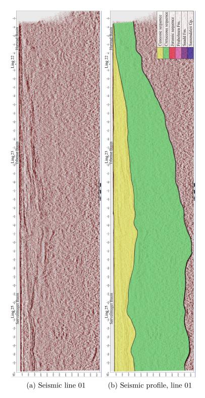
Figure 31: Seismic 2D line 01 and a profile showing the seismic interpretation. The location is shown in Figure 7.
