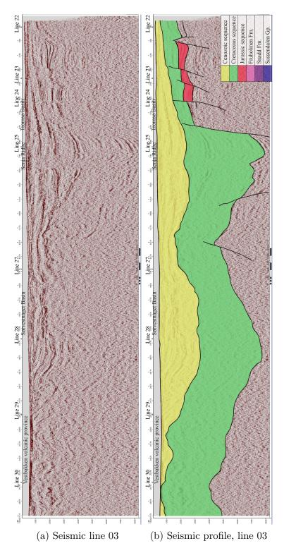
Figure 33: Seismic 2D line 03 and a profile showing the seismic interpretation. The location is shown in Figure 7.
