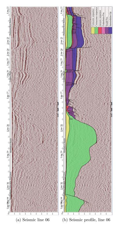
Figure 36: Seismic 2D line 06 and a profile showing the seismic interpretation. The location is shown in Figure 7.
