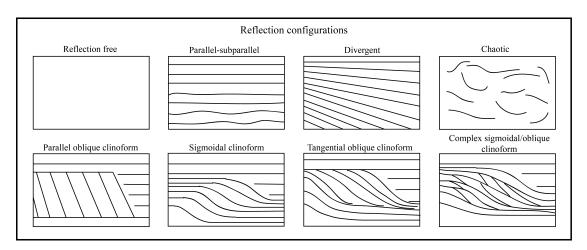
Figure 8: Seismic reflection configurations.
