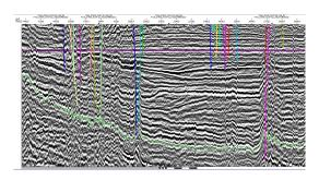
Figure 16: Seismic clinoforms from seismic line 23 showing southwestern progradation. Flattened at Top Sassendalen.
