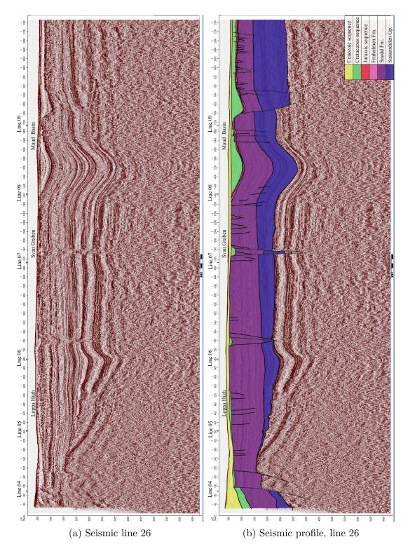
Figure 25: Seismic 2D line 26 and a profile showing the seismic interpretation. The location is shown in Figure 7.
