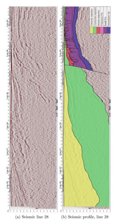
Figure 29: Seismic 2D line 28 and a profile showing the seismic interpretation. The location is shown in Figure 7.
