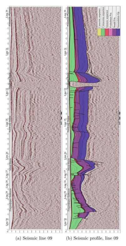
Figure 40: Seismic 2D line 09 and a profile showing the seismic interpretation. The location is shown in Figure 7.
