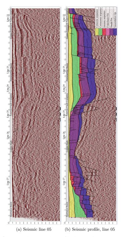
Figure 35: Seismic 2D line 05 and a profile showing the seismic interpretation. The location is shown in Figure 7.
