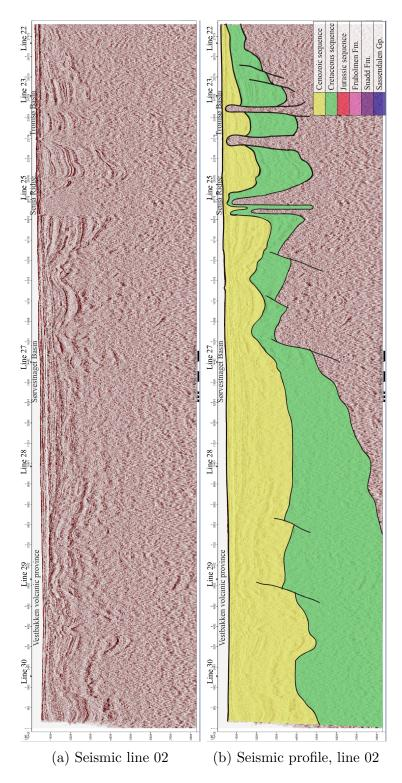
Figure 32: Seismic 2D line 02 and a profile showing the seismic interpretation. The location is shown in Figure 7.
