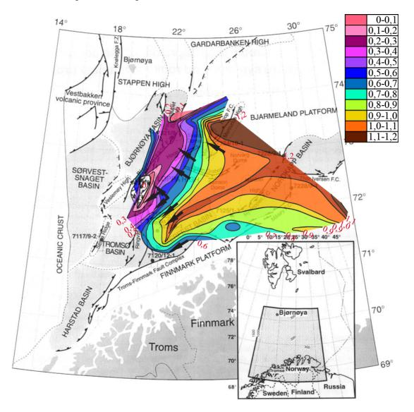
Figure 41: Time-thickness map of the Triassic Sassendalen Group in the study area. The contours are given in seconds. The arrows on the map show the direction of the seismic clinoforms visible on the seismic 2D lines. The structural element map is from Gabrielsen and Kløvjan (1997).
