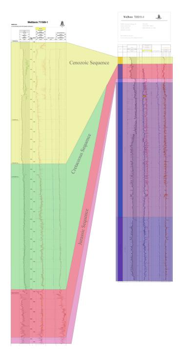
Figure 19: Wells from seismic line 24. Wellbore 7119/9-1 is located at the intersection of seismic line 24 and 03 and wellbore 7222/11-1 is located at the intersection of seismic line 24 and 06. Blue, Sassendalen Group; purple, Snadd Formation; pink, Fruholmen Formation; red, Jurassic; green, Cretaceous; yellow, Cenozoic.
