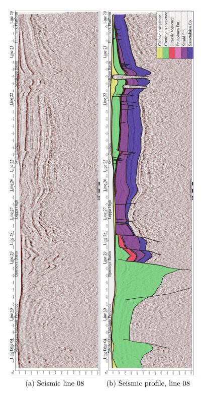
Figure 38: Seismic 2D line 08 and a profile showing the seismic interpretation. The location is shown in Figure 7.
