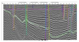
(b) Seismic clinoforms from line 06 in Figure 7. The clinoforms are onlapping the paleo-Loppa High from southeast. Flattened at Top Sassensdalen Group.
