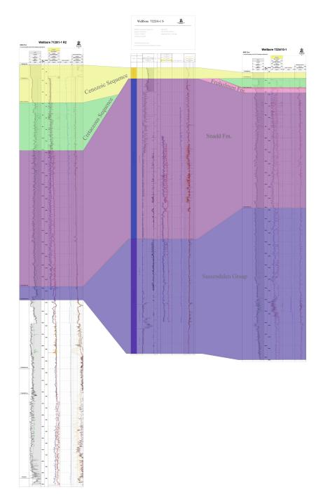
Figure 24: Wells from seismic line 26. Wellbore 7120/1-1R2 is located at the intersection of seismic line 26 and 04, wellbore 7222/6-1S at the intersection of seismic line 26 and 07 and wellbore 7324/10-1 at the intersection of seismic line 26 and 09. Blue, Sassendalen Group; purple, Snadd Formation; pink, Fruholmen Formation; red, Jurassic; green, Cretaceous; yellow, Cenozoic.
