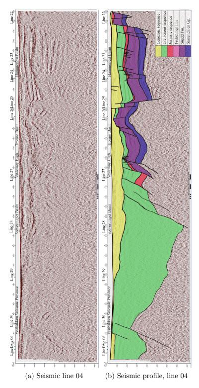
Figure 34: Seismic 2D line 04 and a profile showing the seismic interpretation. The location is shown in Figure 7.
