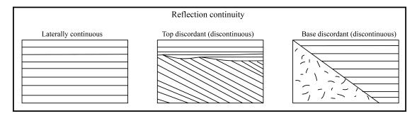
Figure 10: Seismic reflection continuity. Modified from Boggs (2010).
