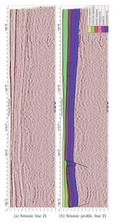
Figure 12: Seismic 2D line 21 and a profile showing the seismic interpretation. The location is shown in Figure 7.
