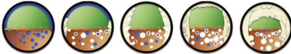
FIGURE 5 CONCEPTUAL ILLUSTRATION OF HYDRATE DEPOSITION ON THE PIPE WALL (SUM 2012).
