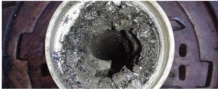
FIGURE 9 EXAMPLES OF HEAVY SCALE PRECIPITATION (STATOIL 2013).
