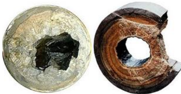
FIGURE 7 EXAMPLES OF HEAVY SCALE PRECIPITATION (STATOIL 2013).
