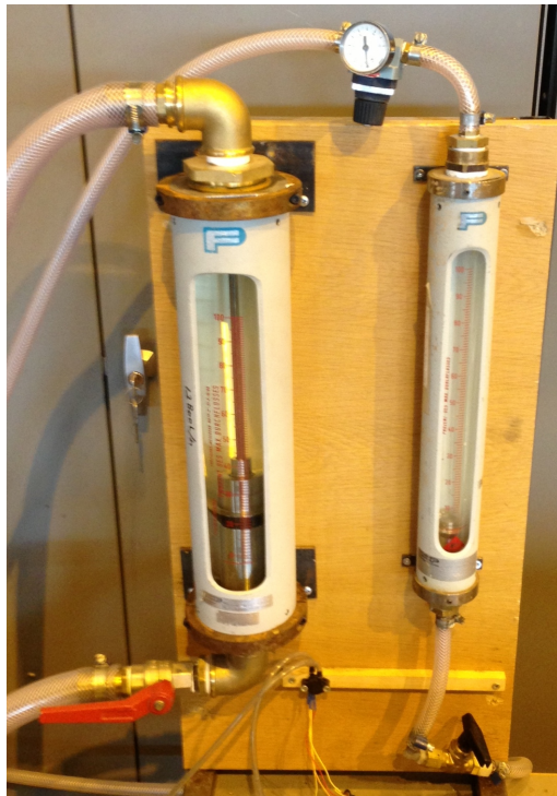
Figure C.4: A close up view of rotameters and the pressure gauge
