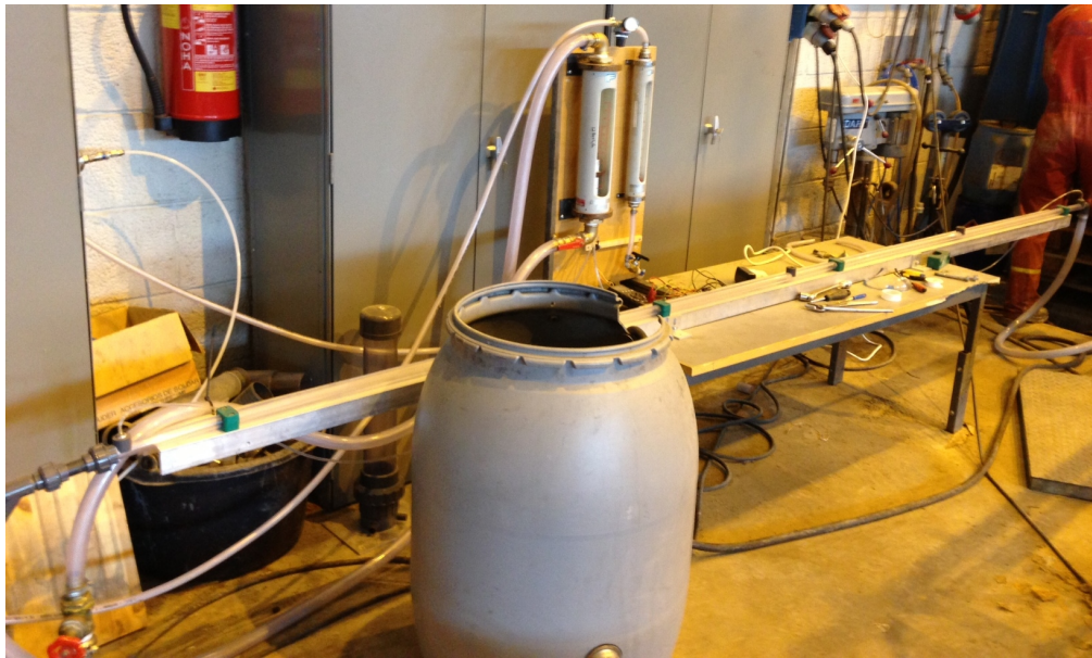
Figure C.2: Experimental setup showing the pipe, the rotameters and the tank
