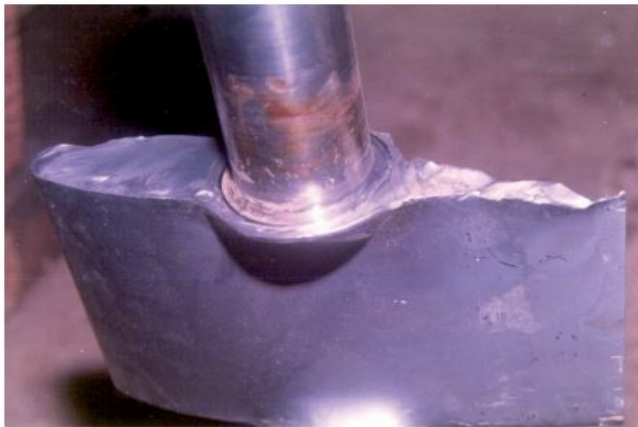
Figure 2.4: Erosion in guide vanes [Gjosaeter, 2011]
