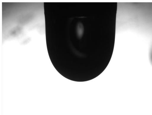
Figure 7.5: Picture of droplet from DropImage Advanced. 20 °C, 90 wt% TEG and 196.6 bar.
