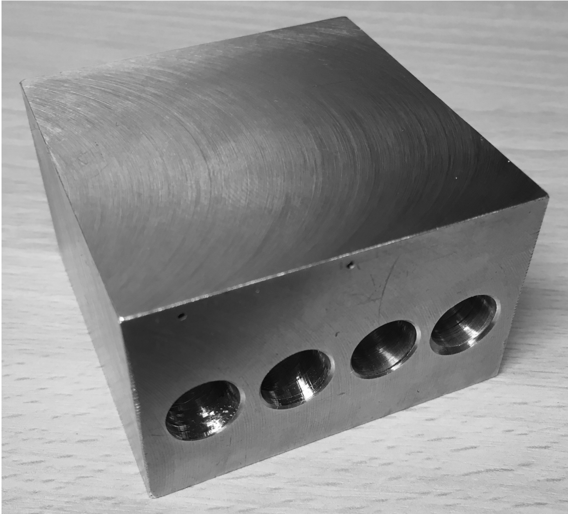
Figure 7.33: Brass block for studying impacting droplets over a micro-nano structure surface, 2" wafers. 4 cartridge heaters (RAC2506-50L10Ø500W , Lojer Components, UK), insulated by 10 mm thick SFC-2 walls (Bagges AS, Norway) and monitored by 3 K-type thermocouples (KMQSS-IM050U-150, Omega, UK). Detailed drawings in Appendix D.
