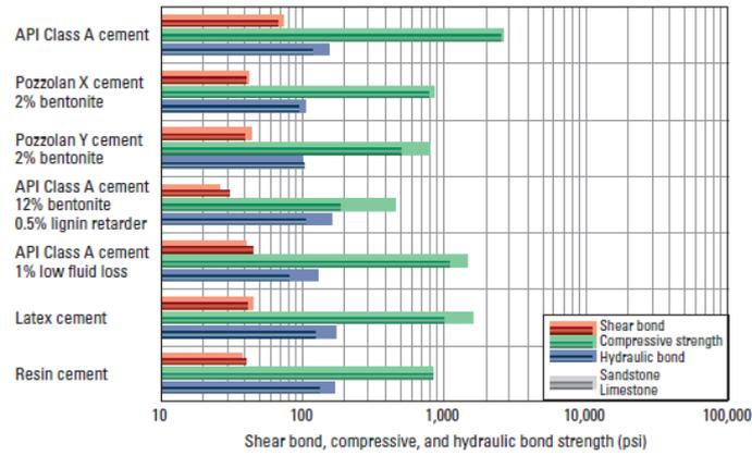
Figure 2-10: Bonding strength of cores with cements not squeezed in presence of mud cake (9).
