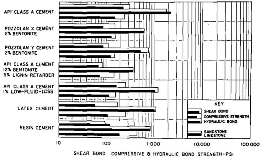
Figure 2-8: Bonding strengths of core against the placement of different muds after the removal of mud cake. Slurry was not squeezed in this case (5).
