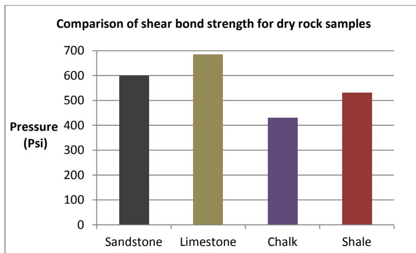
Figure 4-1: Graphical representation of shear bond strength for dry rock samples.
