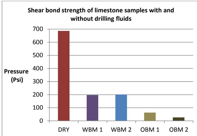
Figure 4-7: Graphical representation of the shear bond strength for limestone samples with and without drilling fluid.
