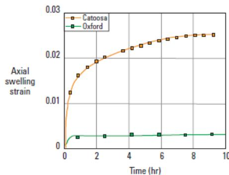
Figure 2-11: Swelling of shale cores in synthetic cement filtrate (6).
