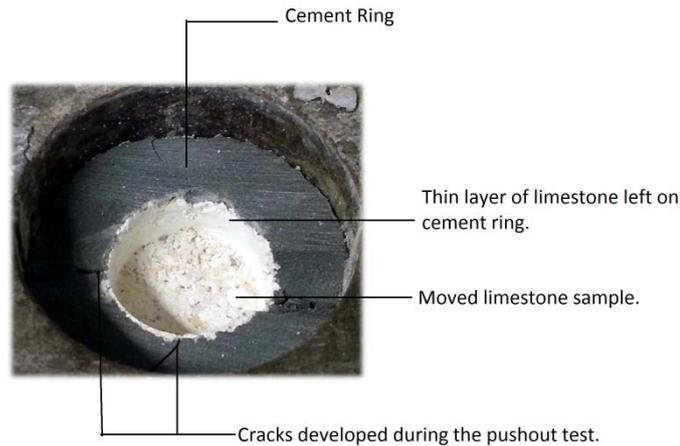
**Figure 4-2: Limestone sample after push-out test showing cracks in the cement and thin layer of limestone inside the cement ring. This shows the failure within limestone sample instead of cement-formation interface.**
