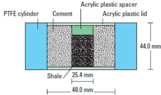
Figure 2-12: Shear bond testing cell with shale formation (6).
