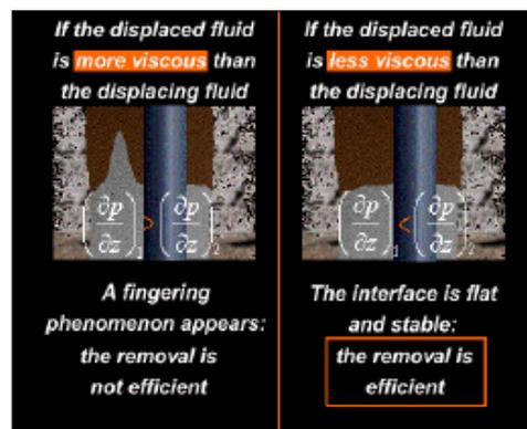
Figure 2-5: Fingering phenomenon caused by using low viscous displacing fluid (left). No fingering effect by using higher viscous displacing fluid (right) (12).
