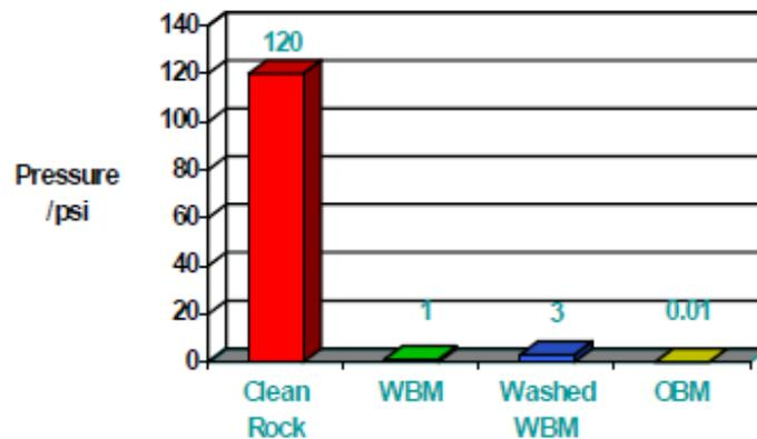
Figure 2-14: Shear bond strength with and without filtercake (6).
