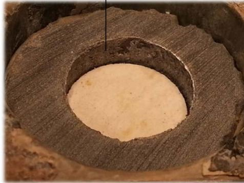
**Figure 4-13: Chalk sample treated with WBM 1 after push-out test. The sample moved along the interface.**
