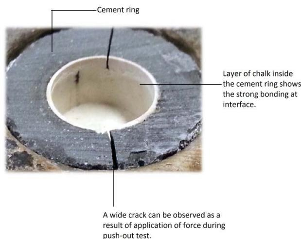
**Figure 4-3: Dry sample of chalk after push-out test. A couple of cracks and a thin layer of chalk are visible inside the cement ring, showing failure within the chalk sample.**
