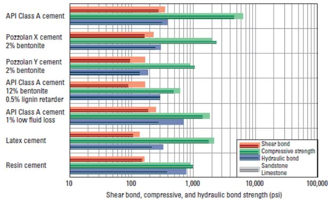
**Figure 2-7: Bonding strength of a core after treatment with water based drilling mud and then placed against different slurries after the removal of mud cake (9).**
