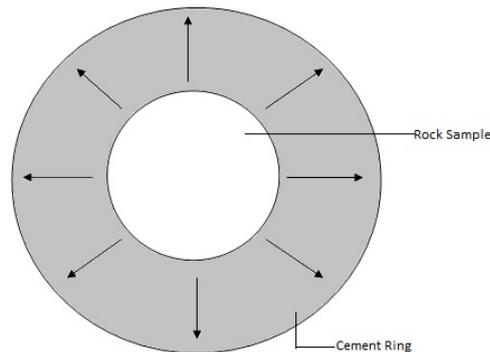
Figure 4-17: Radial stress as a result of applied force during push-out test.
