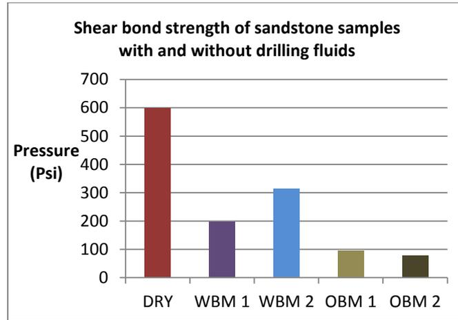
Figure 4-10: Graphical representation of the bond strength of sandstone sample with and without drilling fluids.
