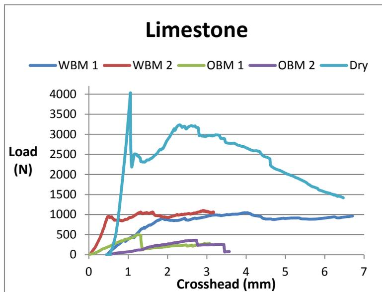
**Figure 4-6:** Graphical representation of data obtained from push-out test. It shows the amount of the force required is increasing to move the rock sample within the cement ring alongwith distance.
