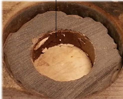
**Figure 4-14: Chalk sample treated with OBM 2. Presence of thin layer of oil constituent reduces its tendency to form strong bond with cement.**
