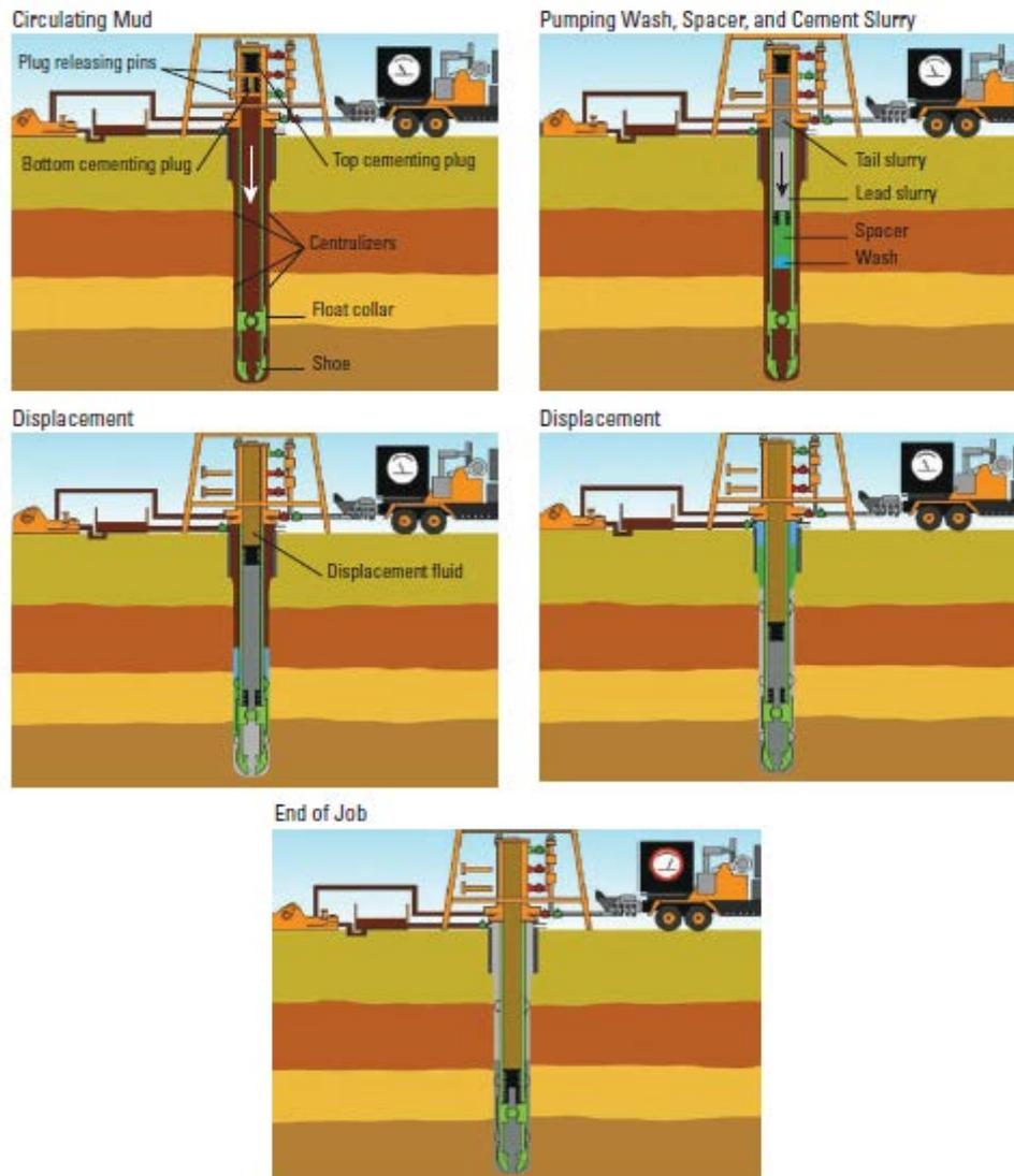
**Figure 2-2: Illustration of different stages for typical primary cementing including circulation of mud, spacers and displacement of cement slurry (9).**
