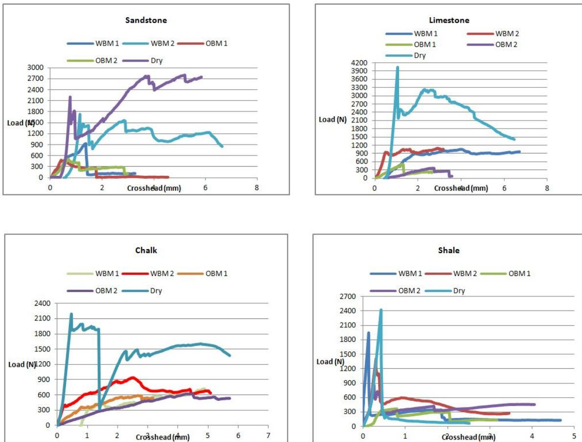
Figure 4-15: Raw data for all rock types from push-out test.
