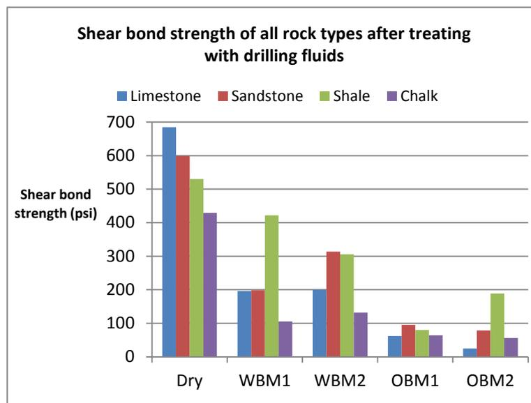
Figure 4-19: Illustration of shear bond strength of all rock types.
