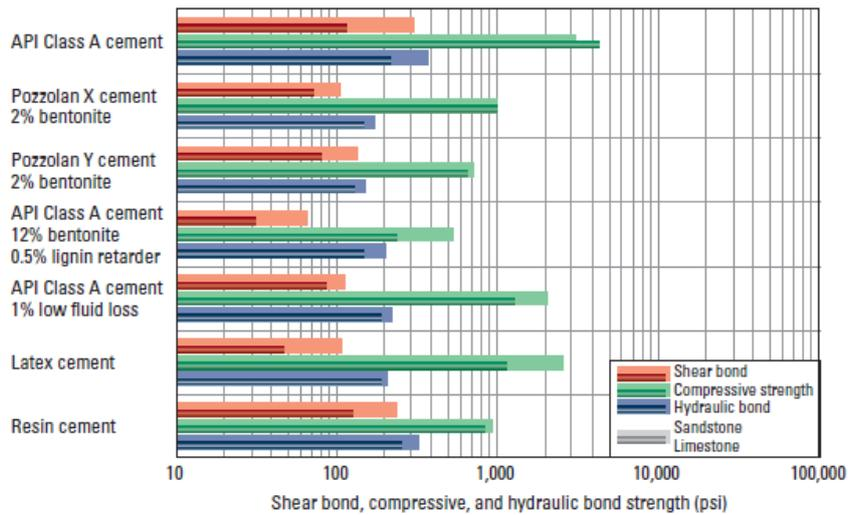
Figure 2-9: Bonding strength of cores with cements squeezed in the presence of mud cake (9).
