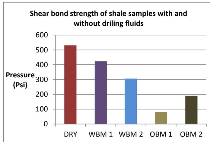
Figure 4-11: Graphical representation of bond strength of shale samples with and without drilling fluid.
