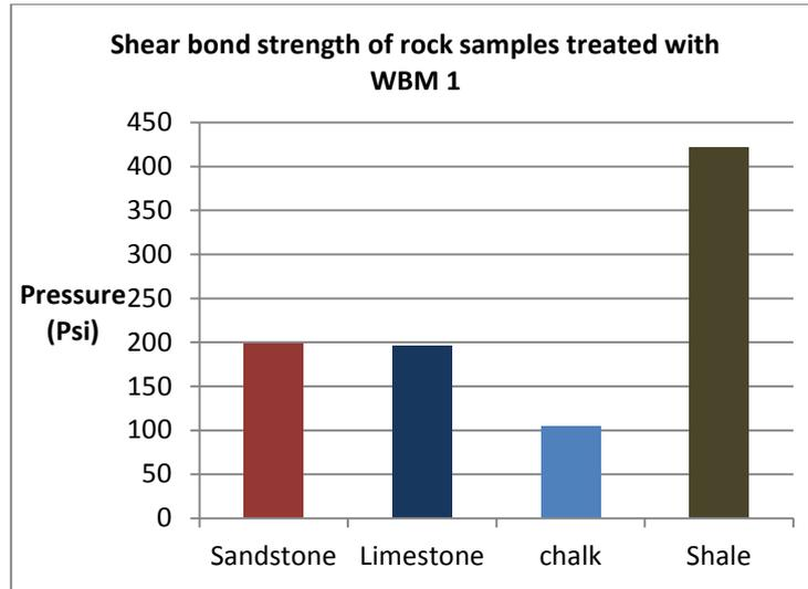
Figure 4-18: Shear bond strength of rock samples treated with WBM1.
