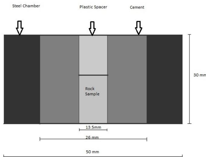
Figure 3-1: Schematic diagram of sample preparation in steel chamber.
