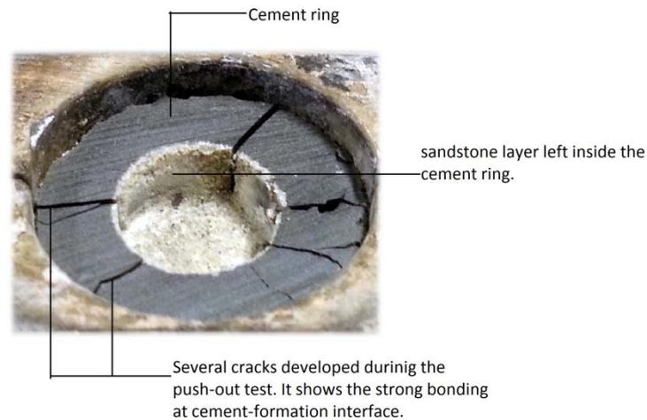
**Figure 4-4: Dry sandstone sample leaving the thin layer inside the cement ring. Several cracks developed as a result of push-out test.**
