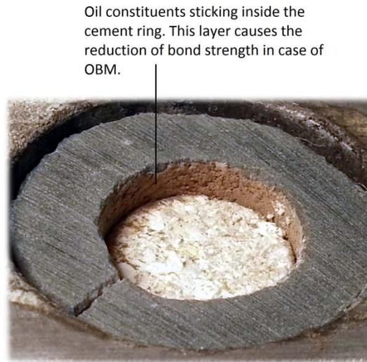
**Figure 4-9: limestone sample treated with OBM 2. Reduction in bond strength is due to the thin film present at the interface.**
