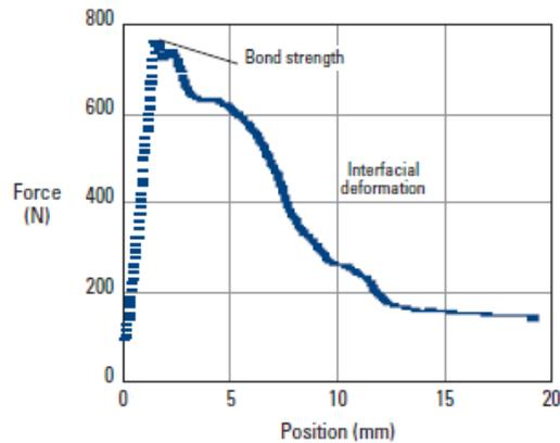
Figure 2-13: The push out profile of Oxford shale from cement (9).
