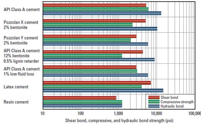
**Figure 2-6: Bonding strength of dry core by cementing with different kinds of slurries (9).**
