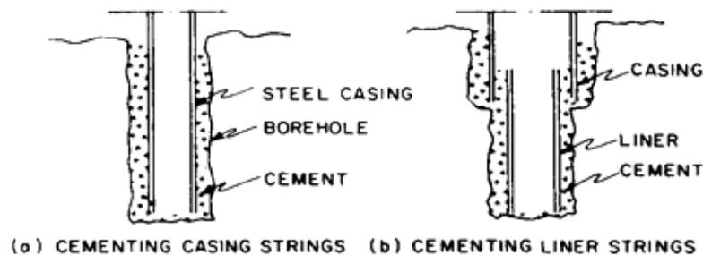
Figure 2-1: Illustration of cement placement in casing and liner string (7).
