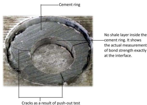
**Figure 4-5: Dry shale sample after push-out test. The shale sample move exactly at shale-cement interface, while some cracks were developed during shale sample movement.**
