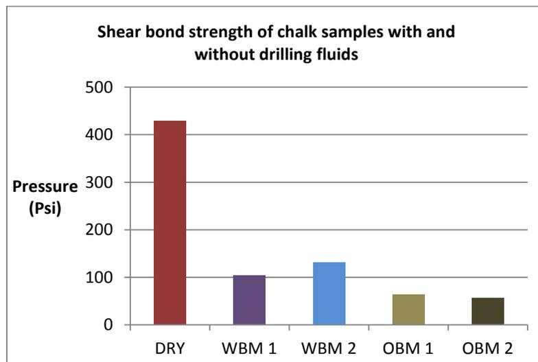
Figure 4-12: Graphical illustration of bond strength of chalk samples with and without drilling fluid.
