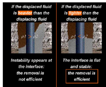
Figure 2-4: Effect of light displacing fluid. It causes improper removal of mud (left). Stable interface is achieved by having dense displacing fluid, results in efficient mud removal (right) (12).
