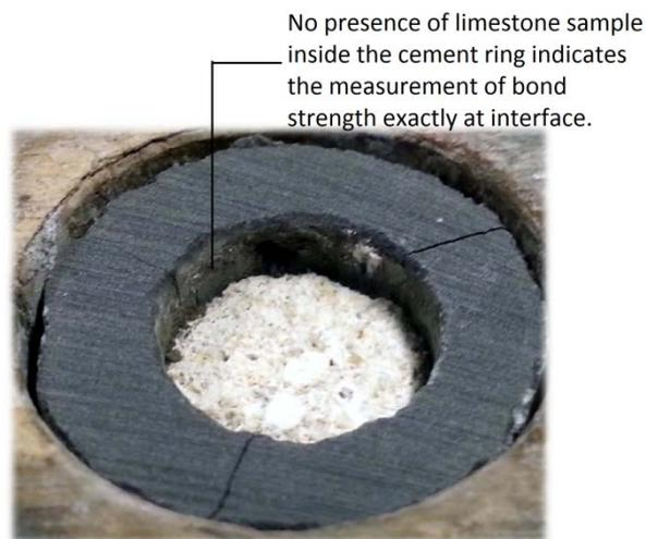
Figure 4-8: Limestone sample treated with WBM 1, showing the measurement of bond strength at interface.
