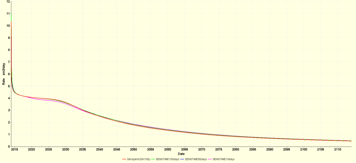
Figure 28: Water production in MORE with diffusion time = 2.5 (red), 10 (green), 50 (blue) and 100 days (purple).
