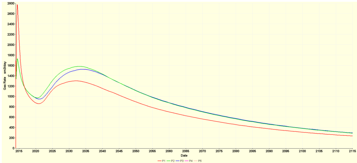
Figure 32: Gas production rate in Eclipse for a five-spot pattern. The wells are P1 (red), P2 (green), P3 (blue), P4 (purple) and P5 (yellow).
