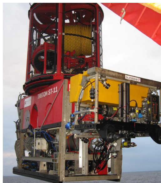
Figure 28: Work ROV Launched From the Seawell [37]
