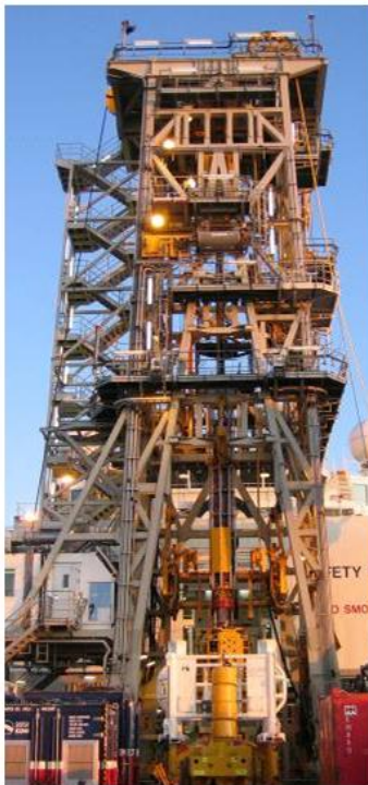
Figure 17: Module Handling Tower [23]
