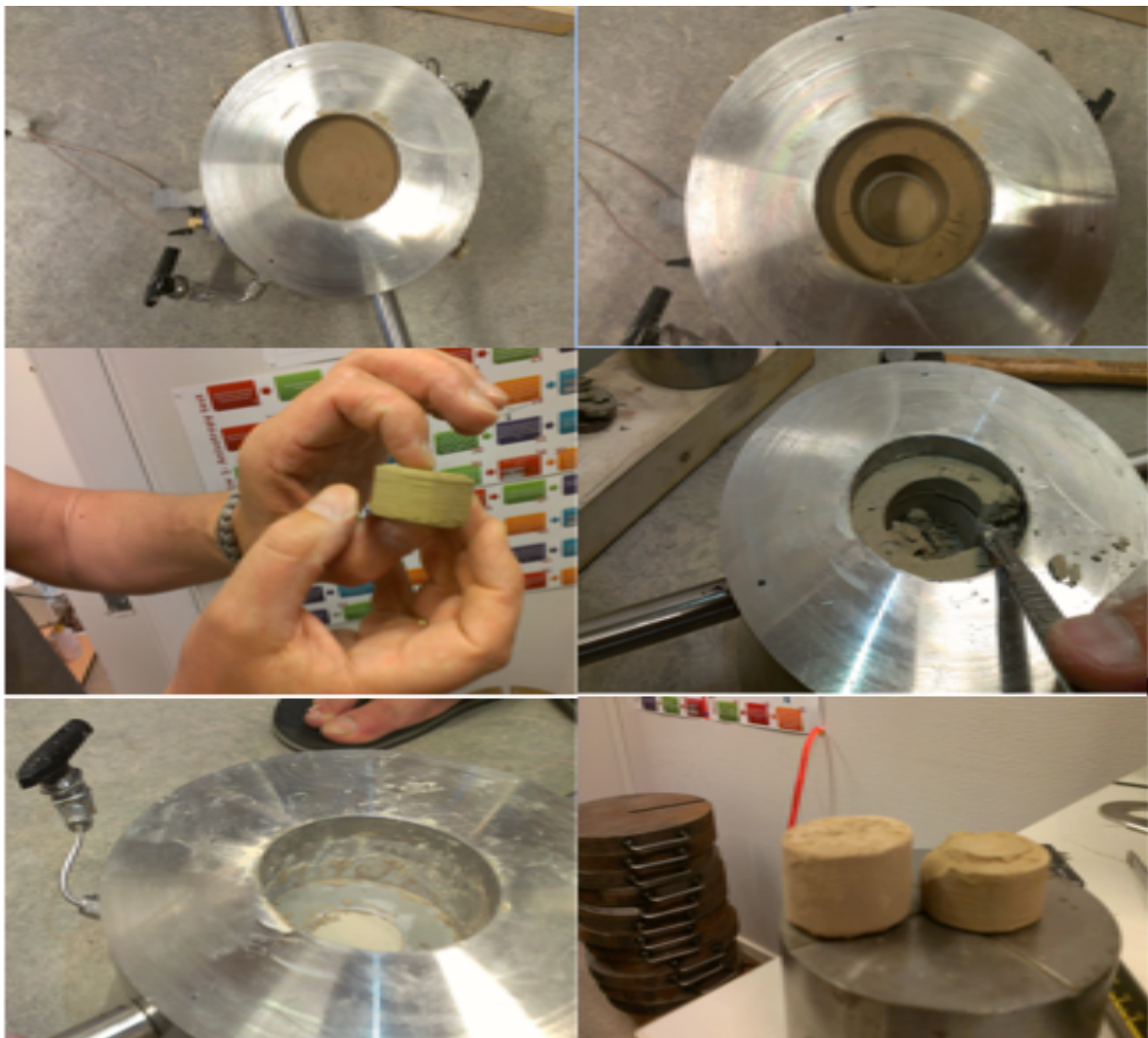
Figure 7.18 Micro-barite sample at the end of the test. The upper left picture shows the sample inside the sample holder. The upper right picture shows the sample when a core of the whole sample is taken out. The middle left picture shows the core. The middle right picture shows a layer in the sample caused by a filling. The lower left picture shows the sample holder walls after the sample is carefully removed. The lower right picture shows the barite and micro-barite core sample.
