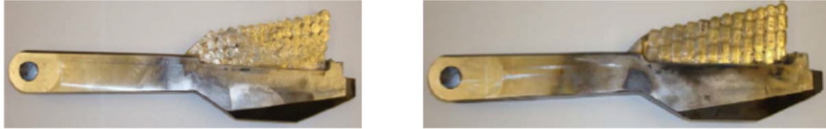
Figure 2.11 Milling blade with traditional cutter and milling blade with new P-Cutter. After (22).
