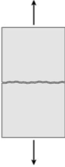
Figure 5.4 Tensile failure. After(36).
