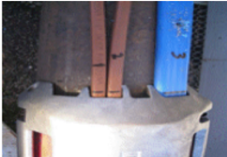
Figure 2.4 Control cables and lines clamped to production tubing. After (5).
