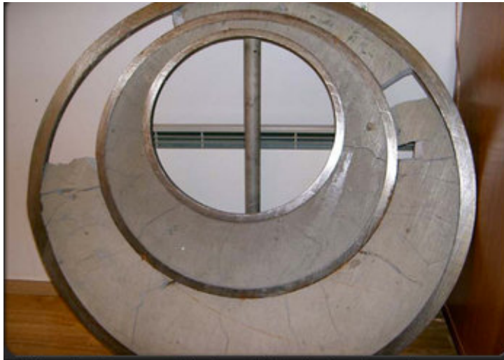
Figure A. 1 Radial cracks in set cement induced by tensile failure as result heat from warm oil flow. After (29).
