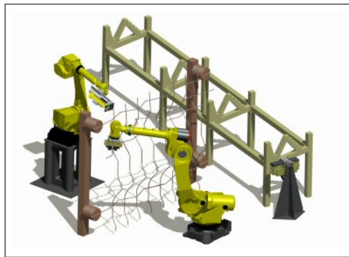
Figure 4.13: Reinforcement production setup prototype [3]
