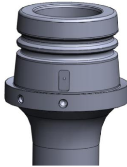
Figure 18: Landing Joint pin head
