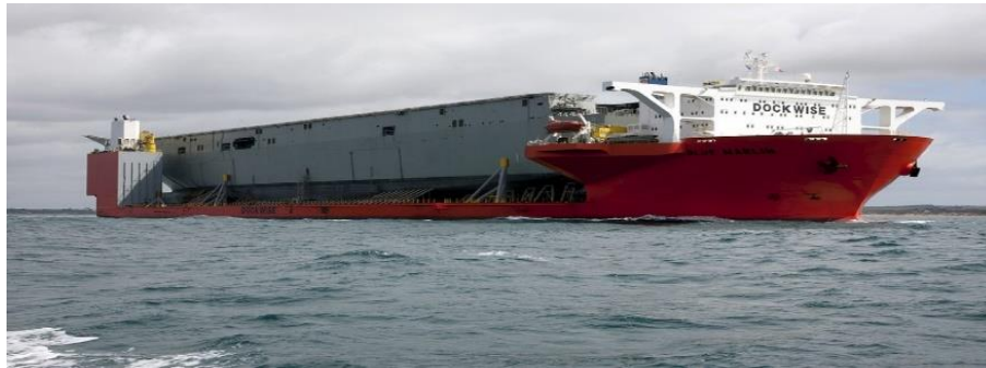
FIGURE 3 - BLUE MARLIN TRANSPORTING THE NAVY VESSEL "CANBERRA" (ELLIOT, 2012)
