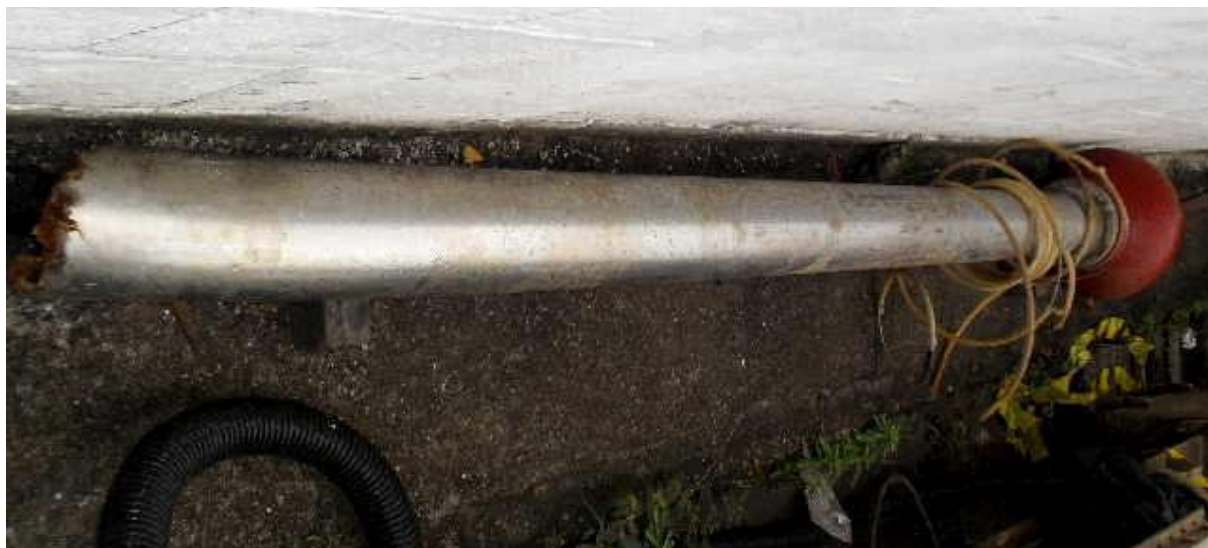
FIGURE 21: THE BROKEN HIPAP 500 TRANSDUCER FROM SKANDI BOTAFOGO (S.A, 2010).
