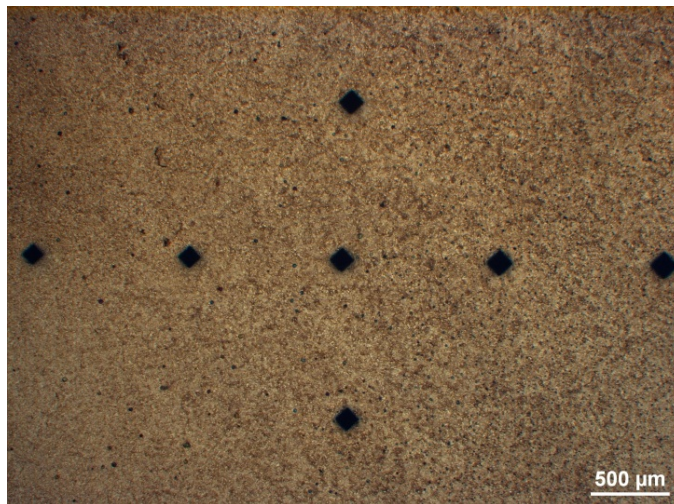
Figure 3-5: Positioning of HV10 indentations in HAZ. Horizontal axis is parallel to length axis of sample.
