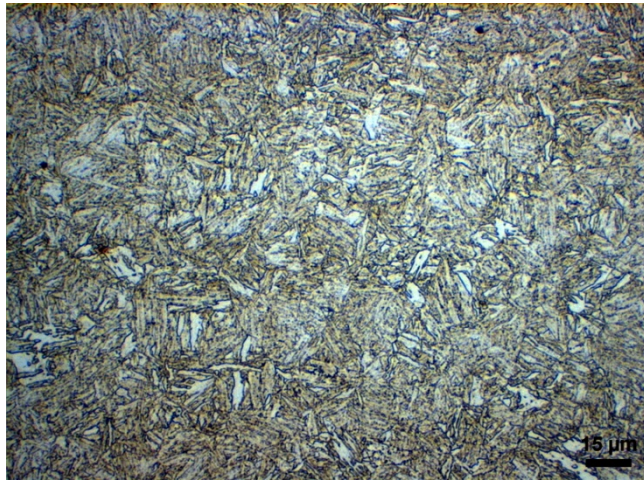
Figure 4-1: Microstructure of C90 prior to weld simulation.
