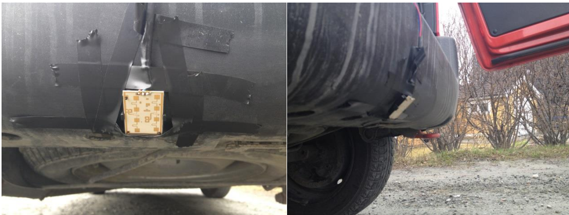
Figure 52 – Radar mounted on the bumper
