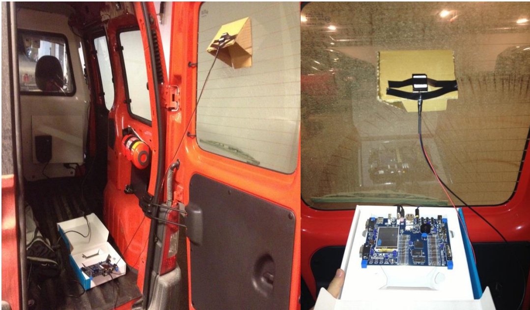
Figure 51 – Radar mounted on the window
