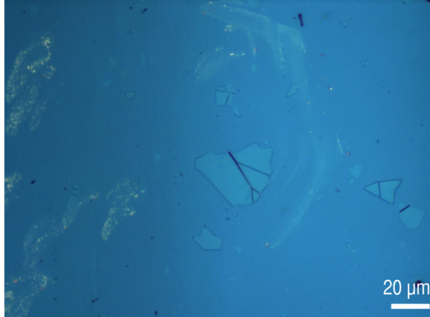
Figure 4.6: An example of a kish graphite sample after the deposition of a thin Al and Si film. The films are uniform and transparent, and kish graphite flakes are clearly visible.
