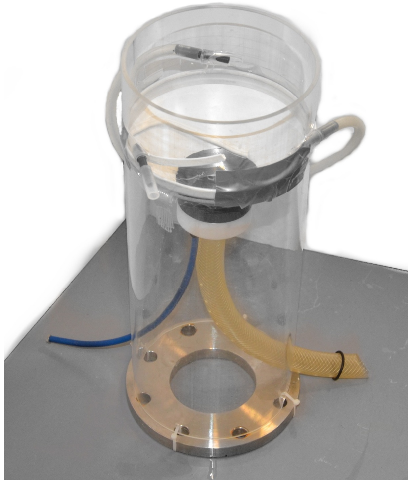
Figure 11.1: Prior art cyclone - This is the prior art cyclone. It consists of a lamp shape, PVC water inlet pipe, and a gardening hose.
