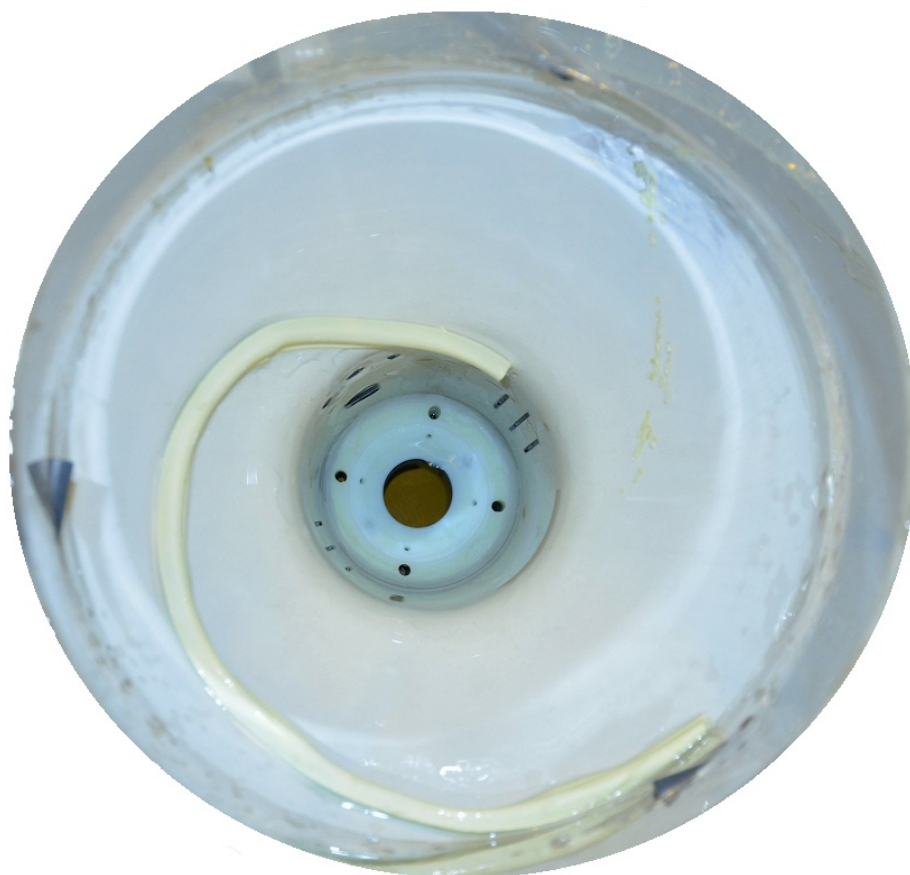
Figure 11.10: Guideline - This is a picture of the prior arts model's whirlpool wall with a guideline. The line helps the speed and direction of water injected in the system.
