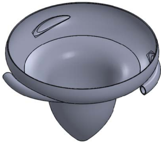
Figure 1: This is a 3D-rendering of the novel innovation. The fish enters in the top of the «bowl». A whirlpool separates the objects that enter and lets them out one at the time.
