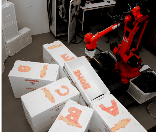
Figure 5.8: Pick-and-place robot - This is the prior art pick-and-place robot created at SINTEF Fisheries and Aquaculture. [Eilertsen (2011)]
