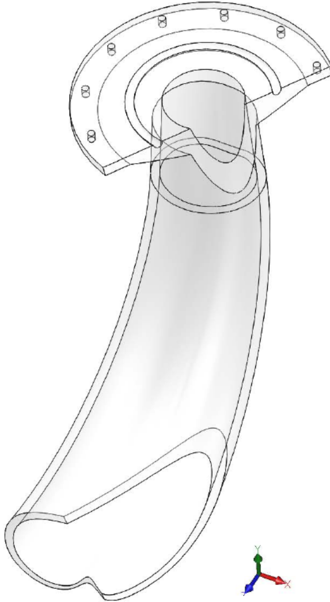
Figure 9.8: The run-off - This is the run-off leading the fish to the input of the weight estimation system. It has a slight split in the middle to ensure that not two fish will lie on top of each other.
