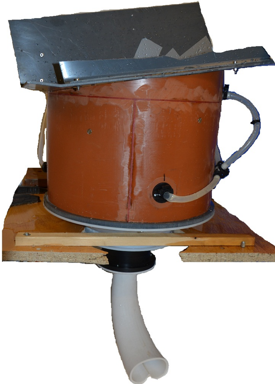
Figure 12.1: The realized conceptual idea - This picture shows the realized conceptual idea, 'the Cyclone'. It is made partially from 3D-printing, and partially by the IME-workshop at NTNU.
