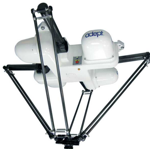
Figure 5.9: Adept Quattro - This is the Adept Quattro, a four legged robot made for high-speed pick-and-place work with high precision. [Quattro (2012)]
