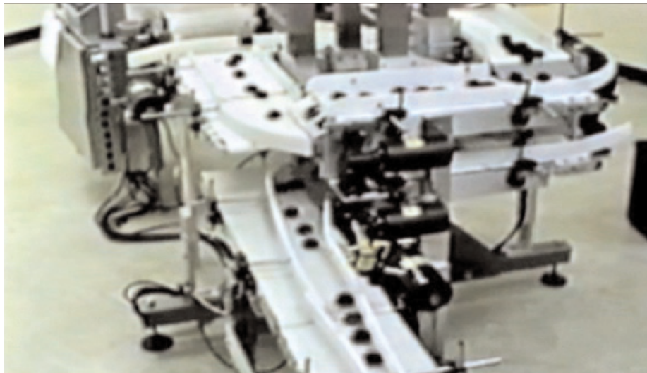
Figure 5.3: Applied Robotics High-speed conveyor belt system - This is an image for a high-speed singulator system created by Applied Robotics.
