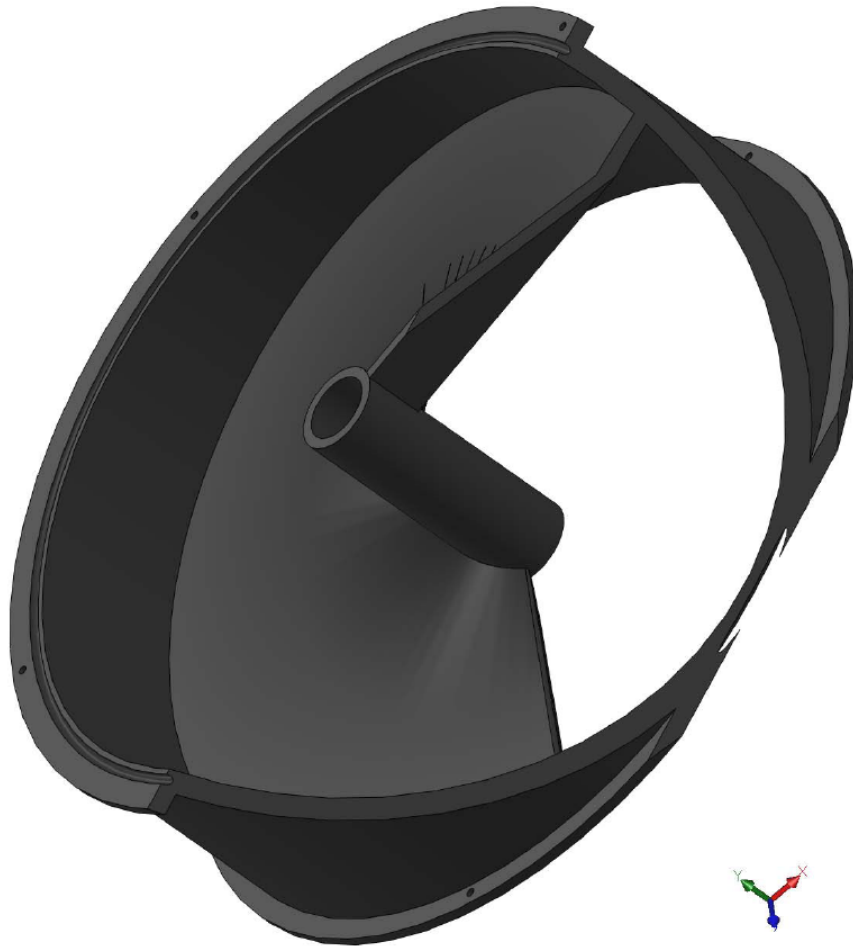
Figure 9.3: The slider - An illustration of the slider employed to ensure that the fish is not dropped into the middle of the system, causing it to jam.
