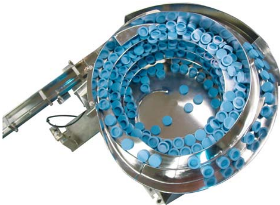
Figure 5.7: Vibration feeder - This is a Singulator that vibrates the whole of its body to exploit friction. [Automation (2012)]
