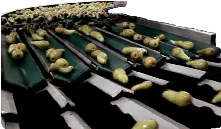
Figure 5.6: Fruit Singulator - Has a set of the conveyor belts moving at different speeds and angles. This machine is made by Burg Machinefabriek. It is defined as a V-belt singulator. [Machinefabriek (2012)]
