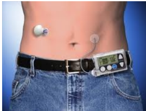
Figure 1.1: Continious blood glucose sensor with insulin pump
