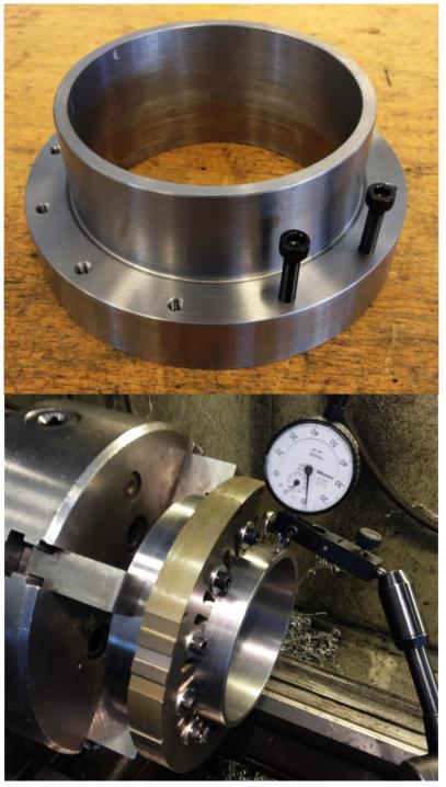
FIGURE 81: STATOR JIG BEFORE AND AFTER MOUNTING IN THE LATHE
