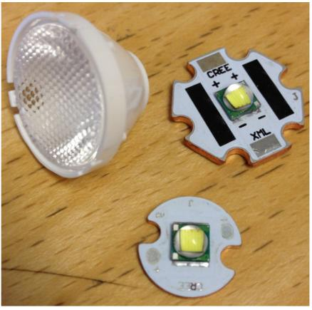
FIGURE 55: 60° LENS (UPPER LEFT), 20MM XML LED (TOP) AND 16MM (BOTTOM)
