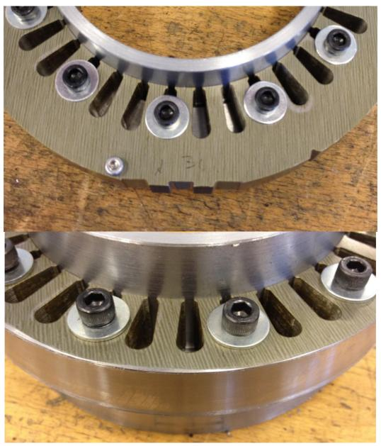
FIGURE 82: THE STATOR IN THE JIG BEFORE (ABOVE) AND AFTER DIAMETER REDUCTION
