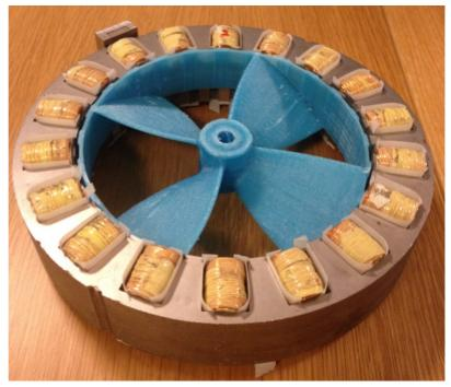
FIGURE 79: SMART MOTOR ACTUATOR STATOR
