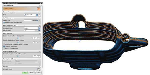
FIGURE 133: HULL FEA 6MM CTETRA(10) MESH
