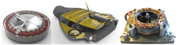
FIGURE 1: LATEST RIM-THRUSTER DESIGN (LEFT) AND FINAL ROV RENDERED WITH A TRANSLUCENT CASING (MIDDLE) AND RIG MOUNTED THRUSTER PROTOTYPE (RIGHT).
