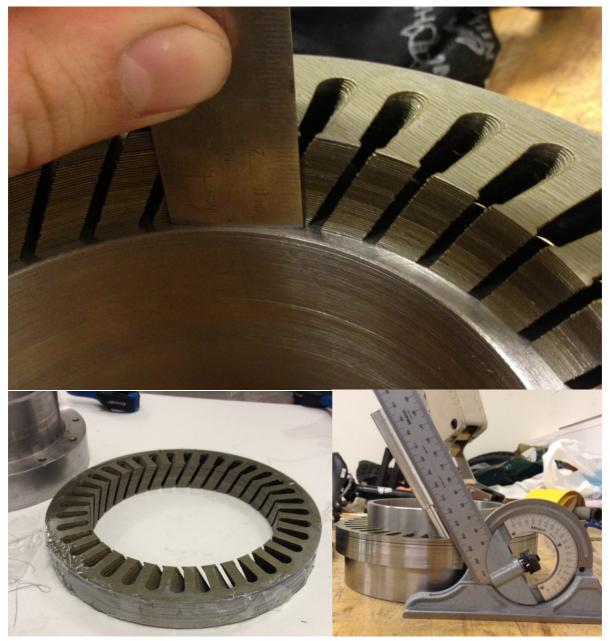
FIGURE 83: SKEWING OF THE STATOR TEETH
