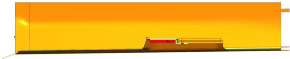
(f) The fixing of the tray will on the back wall consist of studs standing out of the back wall, and nuts fixing the tray onto these
