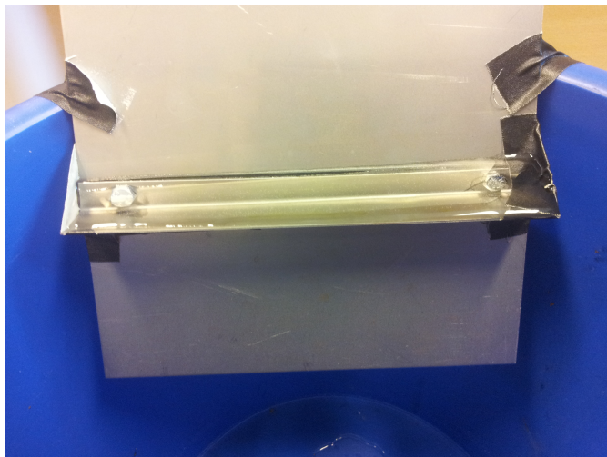
Figure A.16: The neoprene seal test setup after 35min with water.
