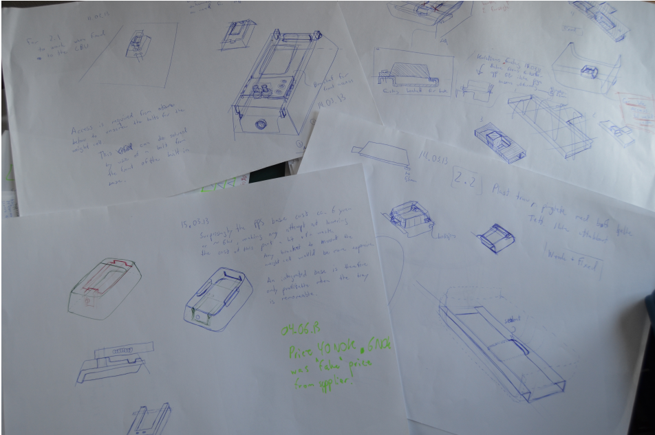
Figure 36: Different concepts for implementing the base into the tray, still enabling the mounting of the weight cell. For a close look see the PU-journal.
