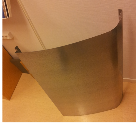
(b) Second upper door prototype 1,25 mm steel. Almost stiff enough even without brackets.
