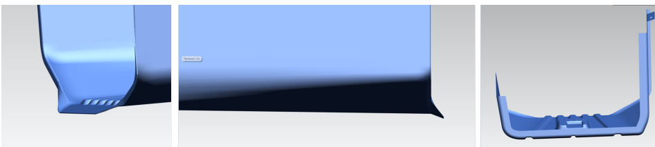
Figure 31: Towards the front of the tray a steep, yet softly blended, 8 mm tall edge forms, ensuring that fluids will not escape elsewhere than into the collection tray in the middle.
