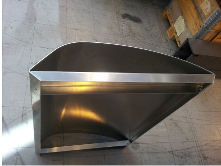
(a) First upper door prototype 2mm aluminium. Not stiff enough.
