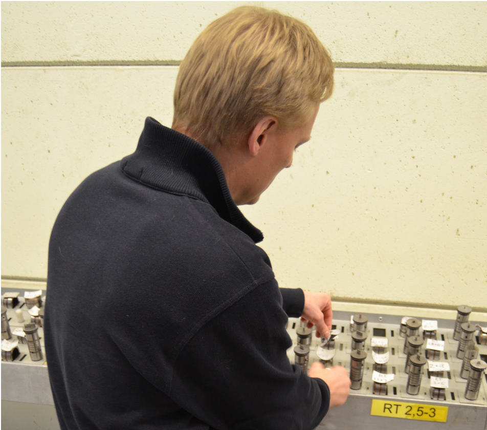
Figure 24: A presentation of different punching tools for revolver puncher at Wermland Mechanics Töckfors AB.
