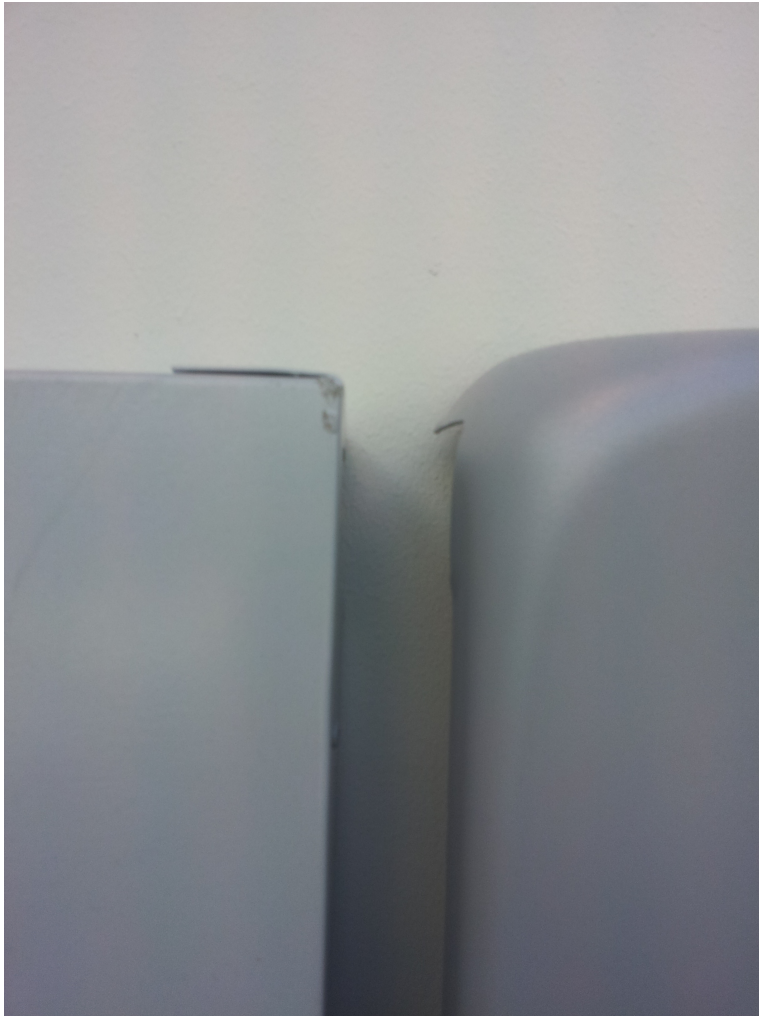
Figure 26: The large radii required for a single step shaping of a closed corner. Left: A sheet metal door punched and bent. Right: A flexformed door concept.
