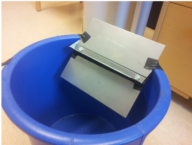
Figure A.15: The neoprene seal test setup.
