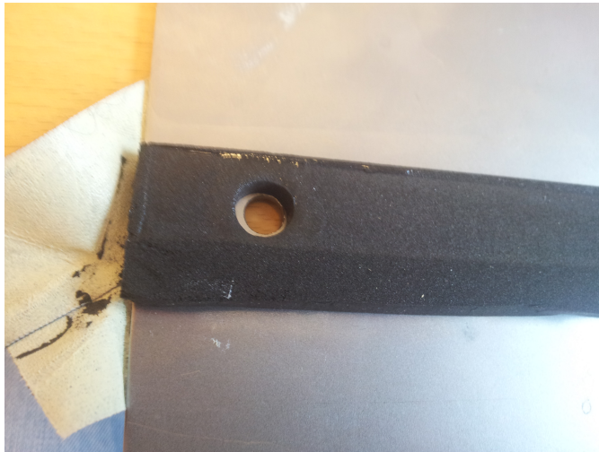
Figure A.18: The neoprene seal after testing, water on the top face.
