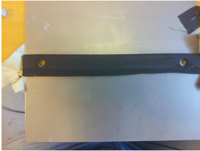
Figure A.17: The neoprene seal after testing, water on the top face and around screw hole.
