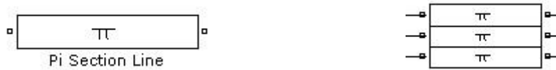
Figure 18 - Pi section blocks in SimPowerSystems. Single phase (left) and three phase (right)
