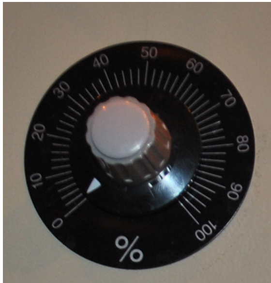
Figure 6.1: The pump flow rate can be adjusted manually from 0-100%.
