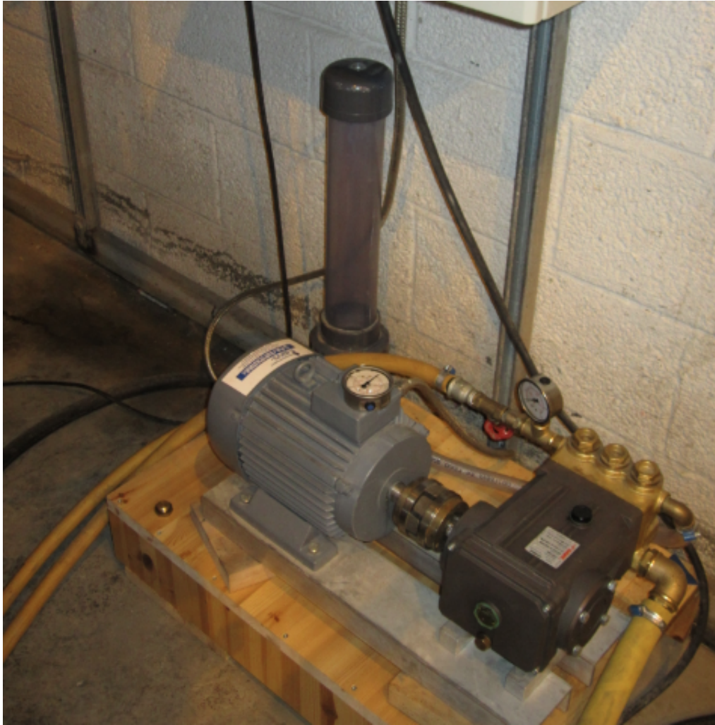
Figure 2.7: Picture of the pump. Also in the picture is the actuator and a defect safety valve.
