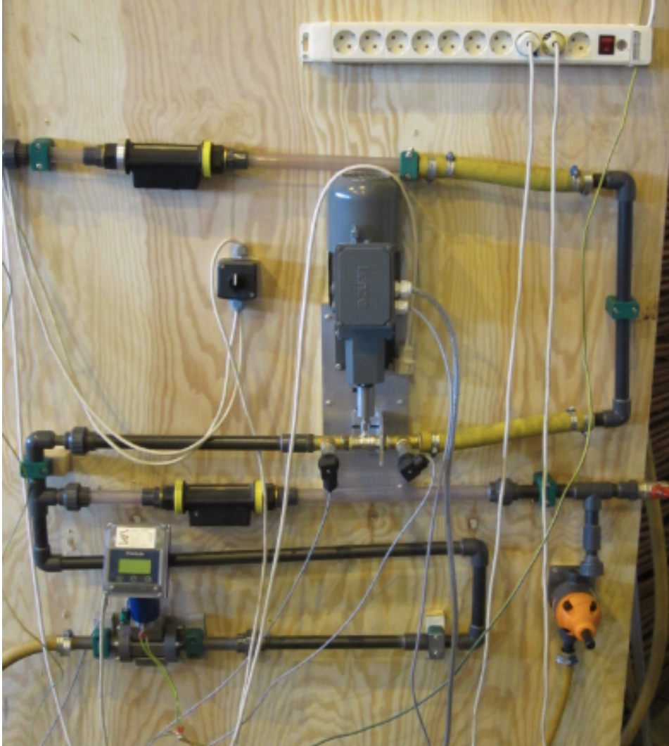
Figure 2.10: Picture of the panel. The pump is connected to the panel from the right. The pipe or by-pass connection can be seen in the lower left corner. The connection downstream the choke is in the left top corner. On the panel there are two gauges, one on each side of the choke, three flow meters and a safety valve.
