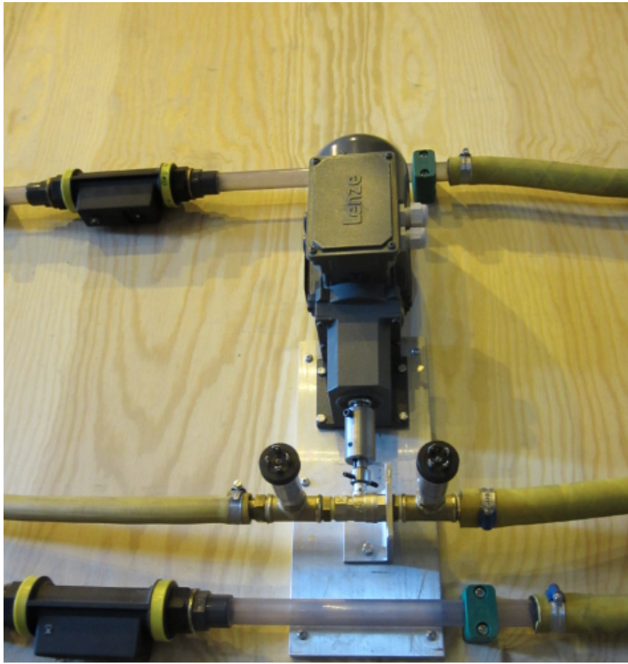
Figure 2.8: Picture of the choke with motor and pressure gauges
