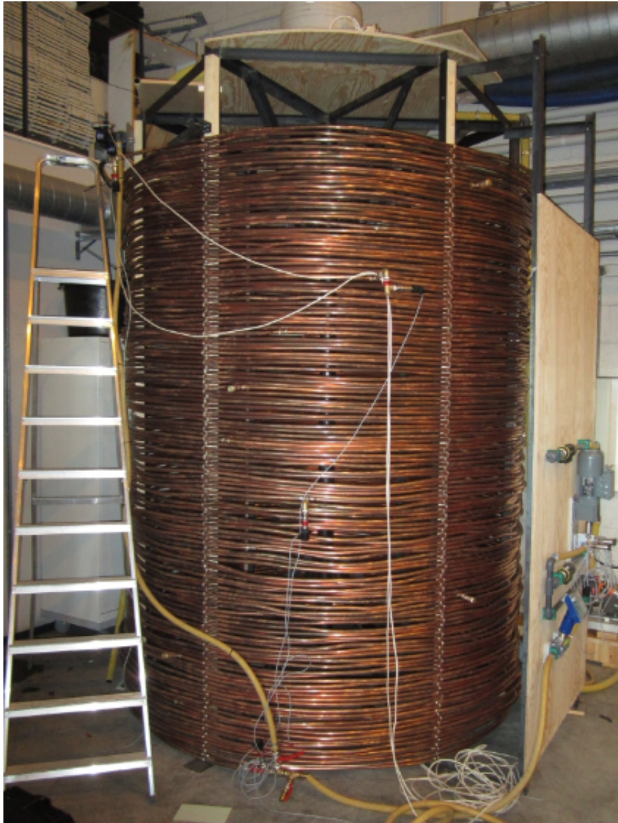
Figure 2.6: Picture of the 900 meter long coiled pipe. As can be seen there are local deviations from the planned curve, in the form of sudden bends. Something that may cause a larger pressure loss than predicted.
