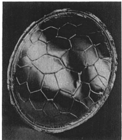
Figure 6-6. Wrinkle Pattern Identified as Turtle Backing of Solid Forward-Domed Rupture Discs Due to Alternate Reverse Flexing and Stretching Against Inadequate Support. (Courtesy of Continental Disc Corporation.)
