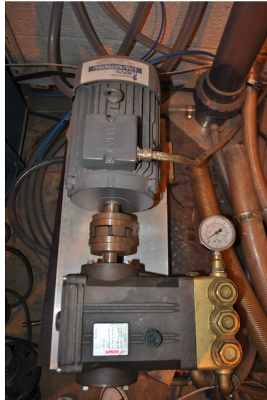
Figure 4.5: The pump system. The mentioned accumulator, which can not be used, can be seen up to the right in the picture.
