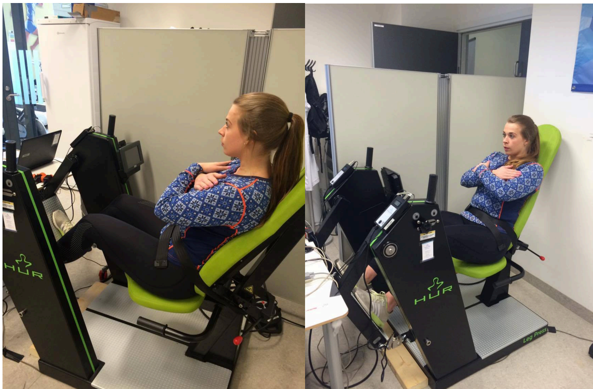
Figure 1. Seated position in HUR isometric leg press. Arms are crossed over the chest, knee angle is 110^{\circ} , and the belt around the hips is fastened (picture used with permission).
