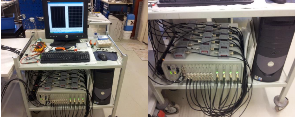
Figure 19. Typical acoustic emission testing system with computer monitoring used in this project.
