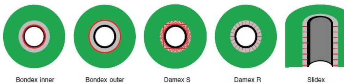
Figure 5. Potential well paths and failures in zonal cement sheath. Represented by debonding between casing and cement, formation and cement, radial cracks, tangential cracks or sliding cracks, (Reddy et al. 2009).
