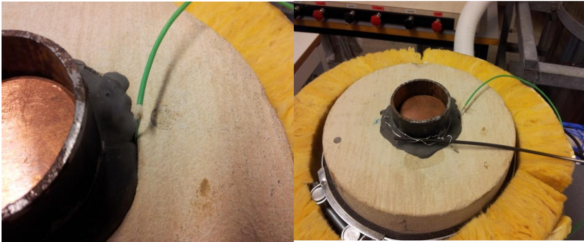
Figure 18. Thermocouples attached to the testing specimen, one at casing and one at cement-formation interface.
