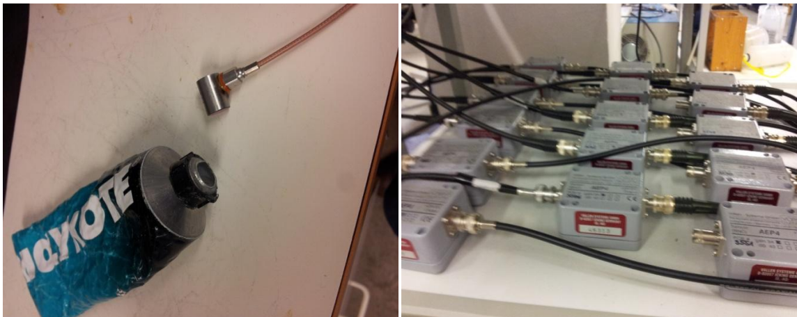
Figure 20. Acoustic emission testing sensor and amplifiers.
